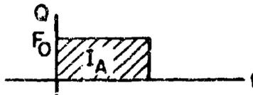
Figure 7. Force-Time Input, Rectangular
