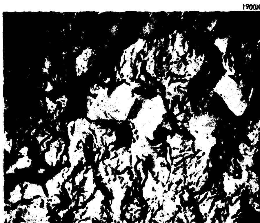
Figure 46 MICROFRACTOGRAPHIC APPEARANCE OF FATIGUE IN 4335M NOTE LOCAL INTERGRANULAR CRACKING
