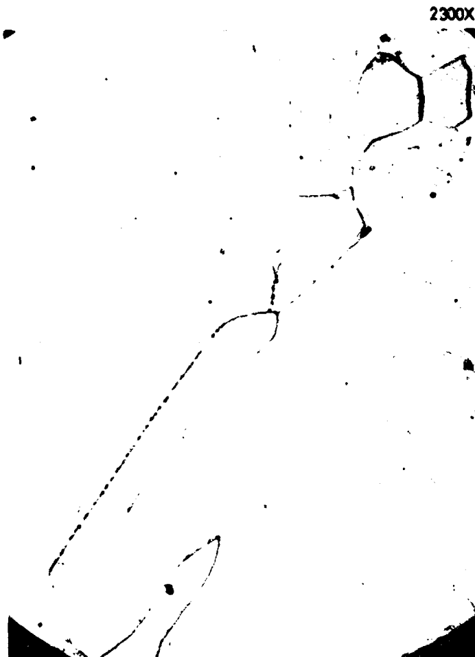
Figure 21 ELECTRON MICROGRAPH OF AM 355 IN THE DADF HEAT TREAT CONDITION NOTE THE ISLANDS OF DELTA FERRITE OUTLINED BY CARBIDES
