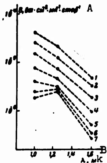
Fig. 4. Spectral relationships in terms of measurements taken on 23 September 1956. Azimuth \xi = 105-150^\circ . 1) H = 6 km; h = 14^\circ ; 2) H = 10 km; h = 16^\circ ; 3) H = 14 km; h = 18^\circ ; 4) H = 18 km; h = 19.5^\circ ; 5) H = 22 km; h = 21^\circ ; 6) H = 26 km; h = 23^\circ ; 7) H = 29 km; h = 24^\circ . A) \text{w} \cdot \text{cm}^{-2} \cdot \mu^{-1} \cdot \text{ster}^{-1} ; B) \mu .
