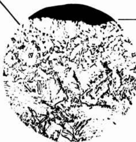
Fig. 101 f MR 3-11-6D8 As Extruded Etch: Krolls Mag: 500X
