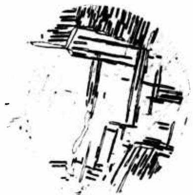
Fig: 98 c MR 4-1-1-G Extruded & Stretch Straightened & STA Etch: Krolls Mag: 500X
