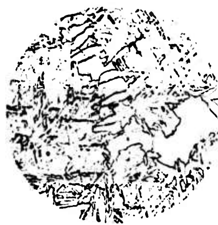
Fig. 97 d MR 4-1-1-C5 As Extruded, Stretch Straightened, Drawn and SS 2 passes plus Age (5)
