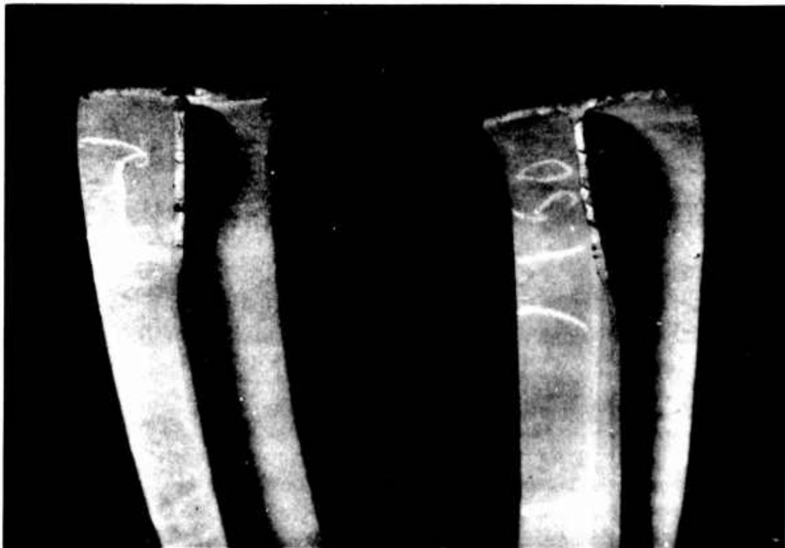
Tears During Initial Break-Through on Extrusion of Cast Billet Material
