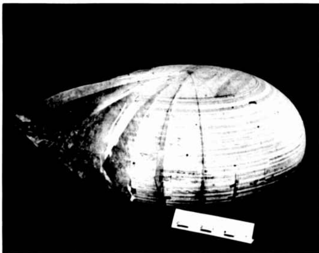
FIG 12-2. MODIFIED 37.5 INCH NOMINAL DIAMETER 10% EXTENDED SKIRT CANOPY FOR OBTAINING GORE AND RIB PATTERN OF GLIDING PARACHUTE
