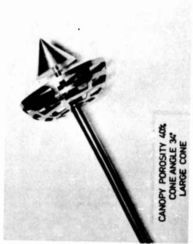
FIG 7-6. RIGID MODEL OF SPIKED RIBBON PARACHUTE
