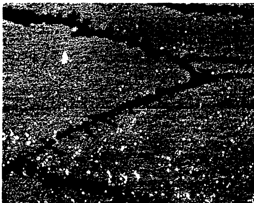
General Structure in Interior of Highly Cracked Area. Etchant - 10% Ammonium persulphate-electrolytic. (500X)
