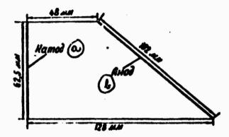
Fig. 4. Diagram of Hull Cell.
