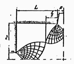
Fig. 5. Diagram to Determine Boundaries of Plastic Zones and Fields of Slip Lines During Stamping With Flow in Two Slots (according to L. A. Shofman). slots, located in mutually-perpendicular planes (in our case slot in mounting and slot in die), found that the magnitude of the extent of the plastic zone de-
