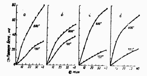
Fig. 7. Reduction of lead agglomerates from Elektrotsink (a), Leninogorsk (b), Ust<sup>\*</sup>-Kamenogorsk (c), and Chimkent (d) Plants with carbon monoxide. 1) Loss in weight; 2) min.
