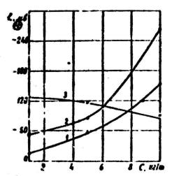
Fig. 3. Effect of acid treatment on electrokinetic potential of pyrochlore I. 1) HF; 2) HCl; 3) H<sub>2</sub>SO<sub>4</sub>; 4) mv.
