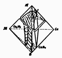
Fig. 4. Lead angle isotherm at 400°C of the Pb-B1-Ca-Sb system.
