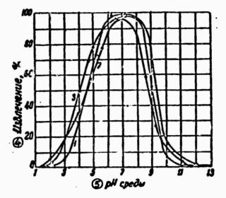
Fig. 3. Influence of pH of medium on extraction of minerals at an oleic acid concentration of 33.3 mg/(.1)Tantalite; 2) tourmaline; 3) garnet; 4) extraction, %; 5) pH of medium.
