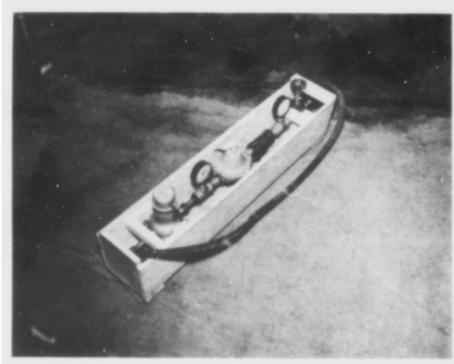
Figure II - Photo of assembled control case. From left to right, the parts are: flow meter, pressure gauge for regulated pressure, adjustable automatic pressure regulator, line strainer, pressure gauge for line pressure, and inlet valve.
