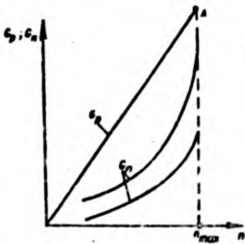
Fig. 227. Available fuel flow rate G_p from gear pump and required fuel flow rate G_r as functions of rotor speed n .
