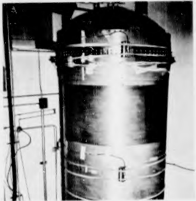
Figure 59. TU-228 Case in Hydrotest Facility
