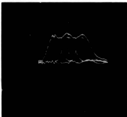
FIGURE 31. Summation of Three Pulses.
