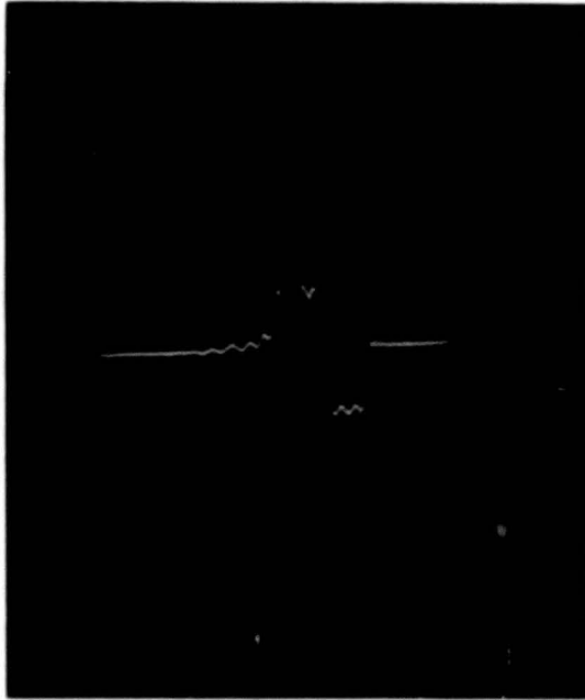
FIGURE 33. Impulse Response of Matched Filter.
