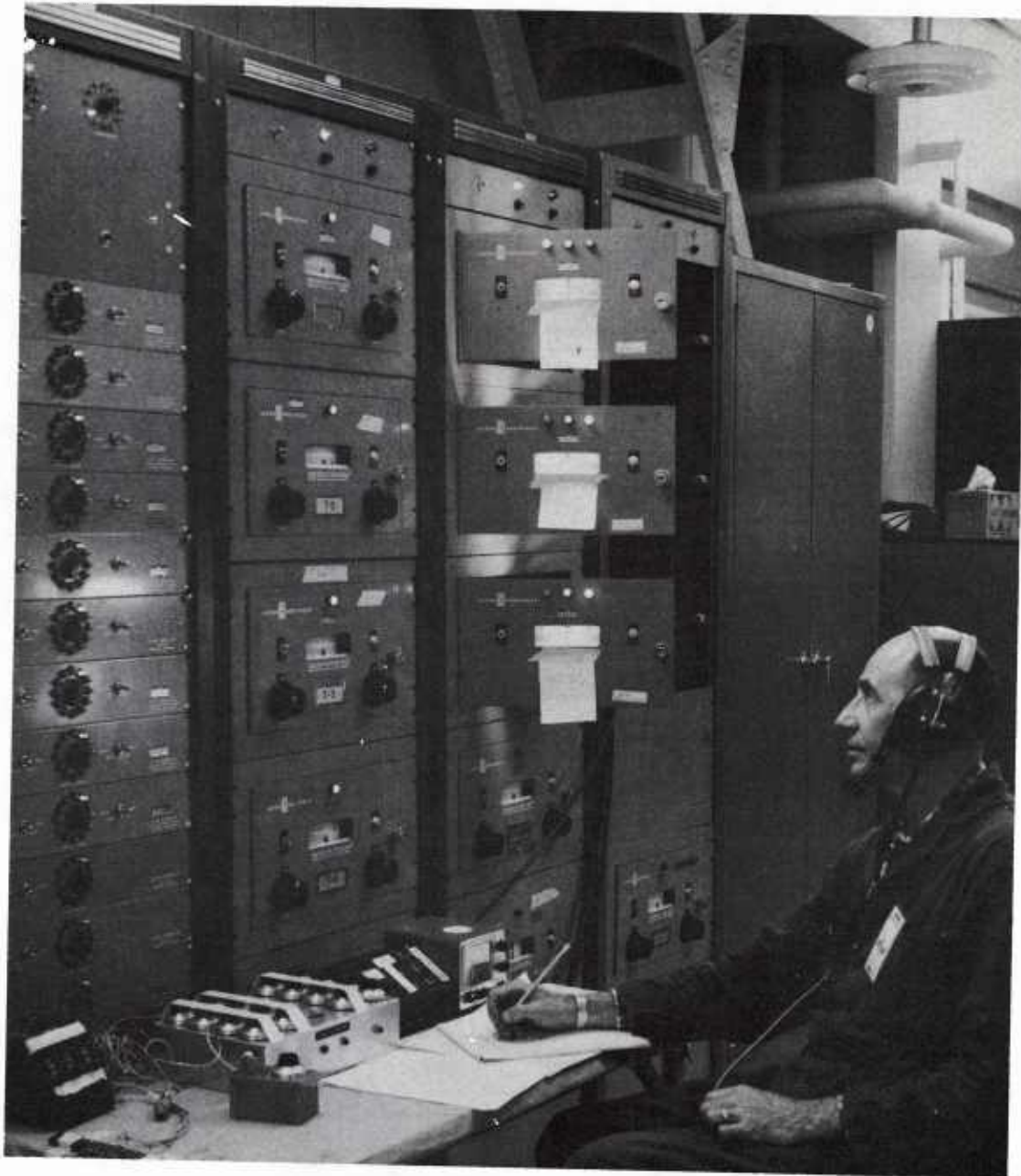
Fig. 6 Photograph of Flap Control and Indicator Panels
