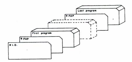
When requesting off-line punching from the FAP Tape, the number of files to be punched should be one greater than the number of programs, since a file mark precedes the first program.
