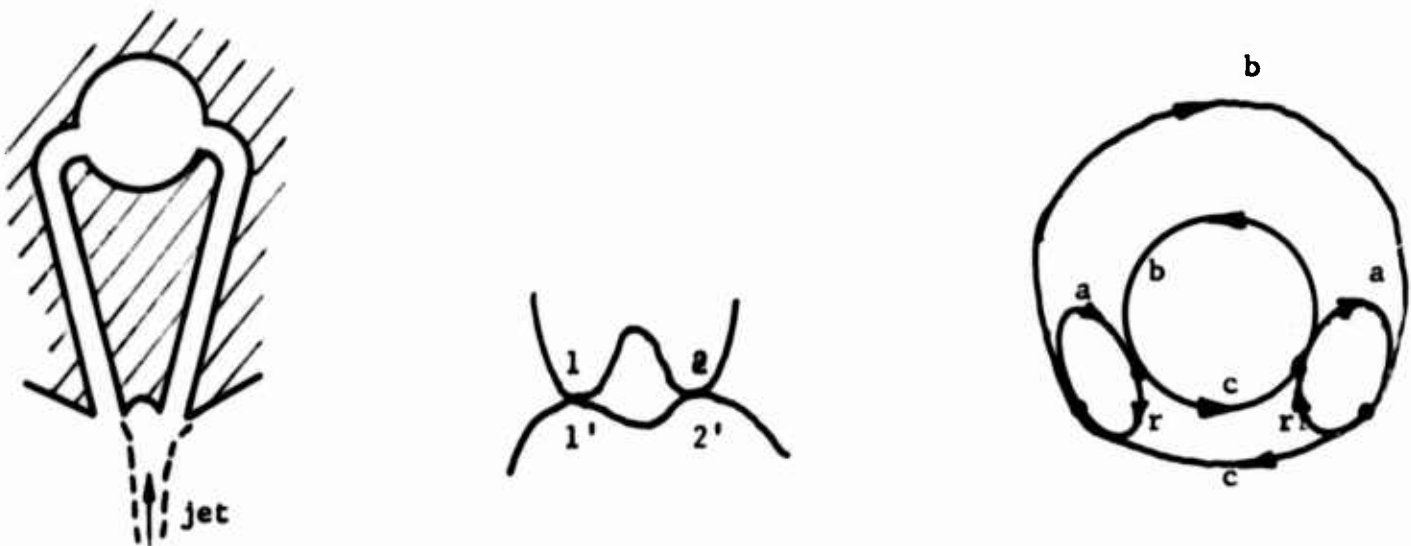
(c) Application as fluid amplifier load, with multiport model and signal-flow graph
