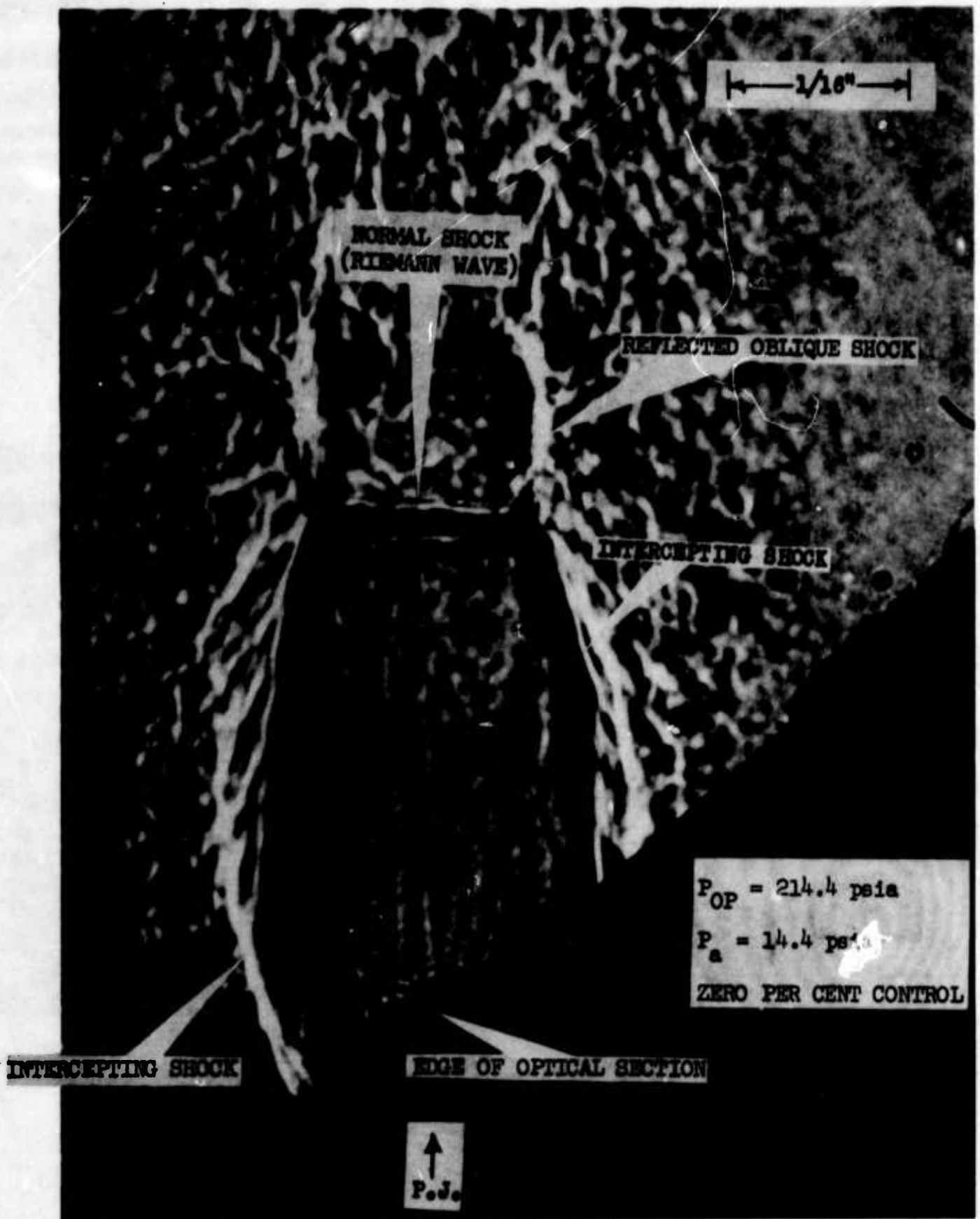
FIG. 2. SHADOWGRAPH OF HIGHLY UNDEREXPANDED TWO-DIMENSIONAL POWER JET FLOW
