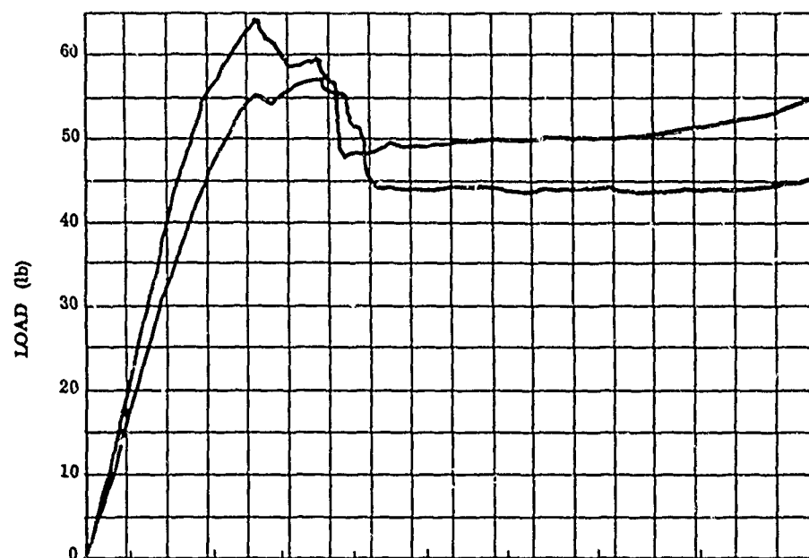
TYPICAL LOAD DEFLECTION CURVE OF A COATED ALLOY IN BEND TESTING
