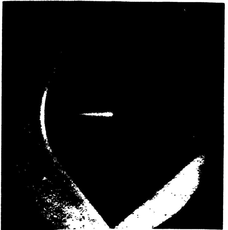
Fig. 17 Schlieren photograph of 50° cone-hemisphere in Mach 10 nozzle, T_5 = 4000^\circ\text{K} .
