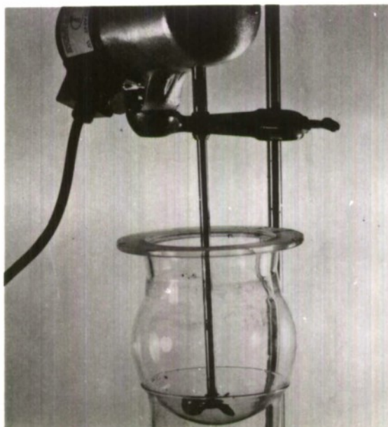
2(c) 'LIGHTNIN' MIXER WITH SPHERICAL VESSEL.
