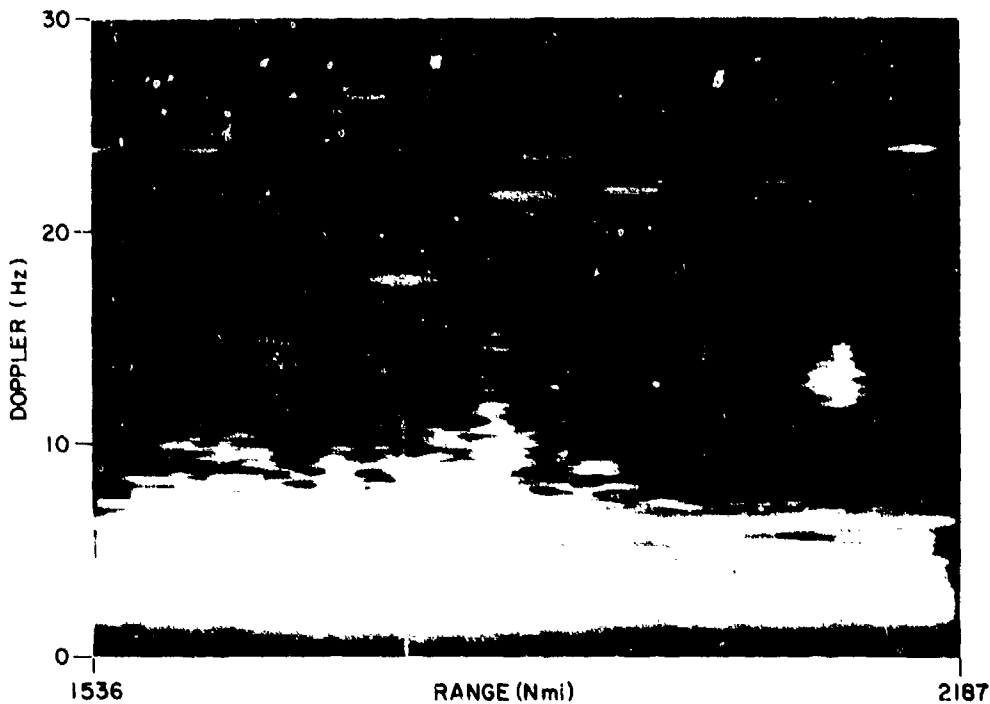
Fig. 2 (S)—Doppler-vs-range display at 170400 GMT with multiple aircraft in view
