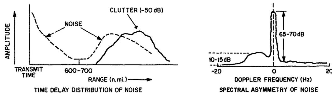
(S) Fig. 1—Description of noise detected with the FPS-95 radar (a) Time-delay distribution of the noise showing the basis for the names clutter-related noise (CRN) and range-related noise (RRN) (b) Spectral asymmetry of the noise
