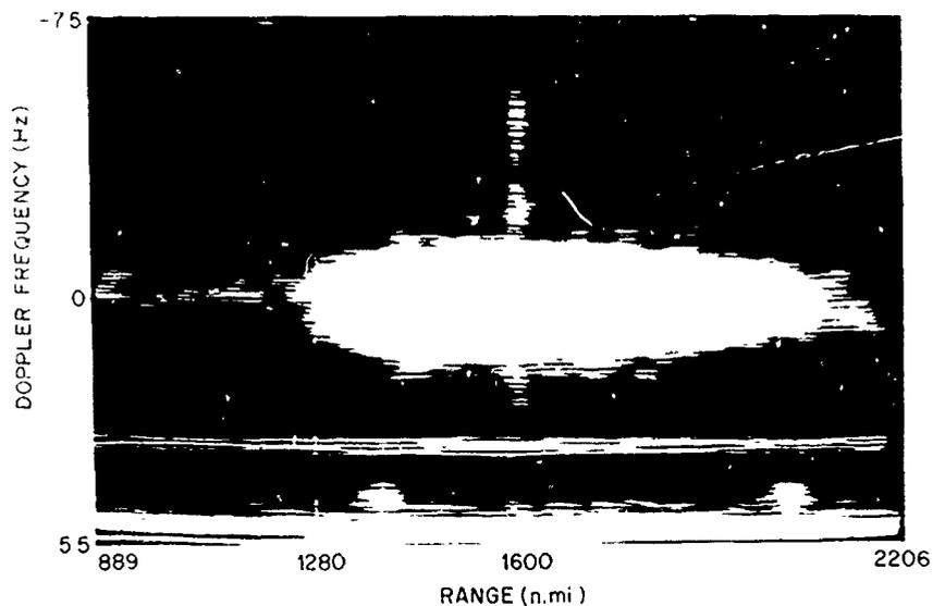
(S) Fig. 13—An offset 5-second doppler-versus-range record showing a far-range meteor echo along with earth return
