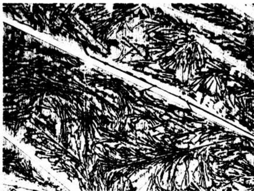
Figure 49. Hf-Si-B: 52/28/20. Arc Melted
