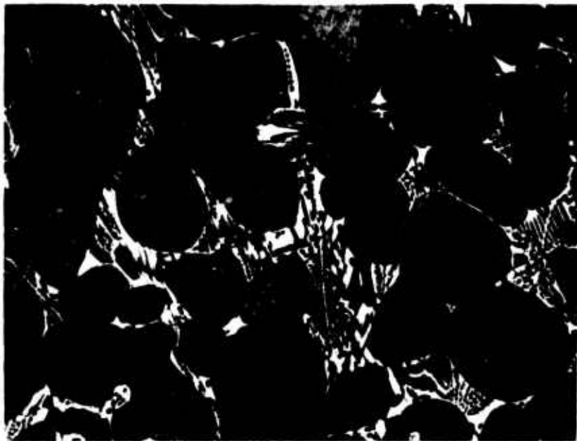
Figure 30. Hf-Si-C: 90/5/5, Quenched from 1908°C.
