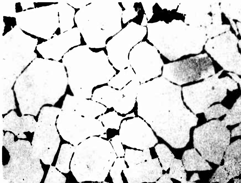
Figure 41. Zr-Si-B: 36/4/60, Quenched from 2847°C
