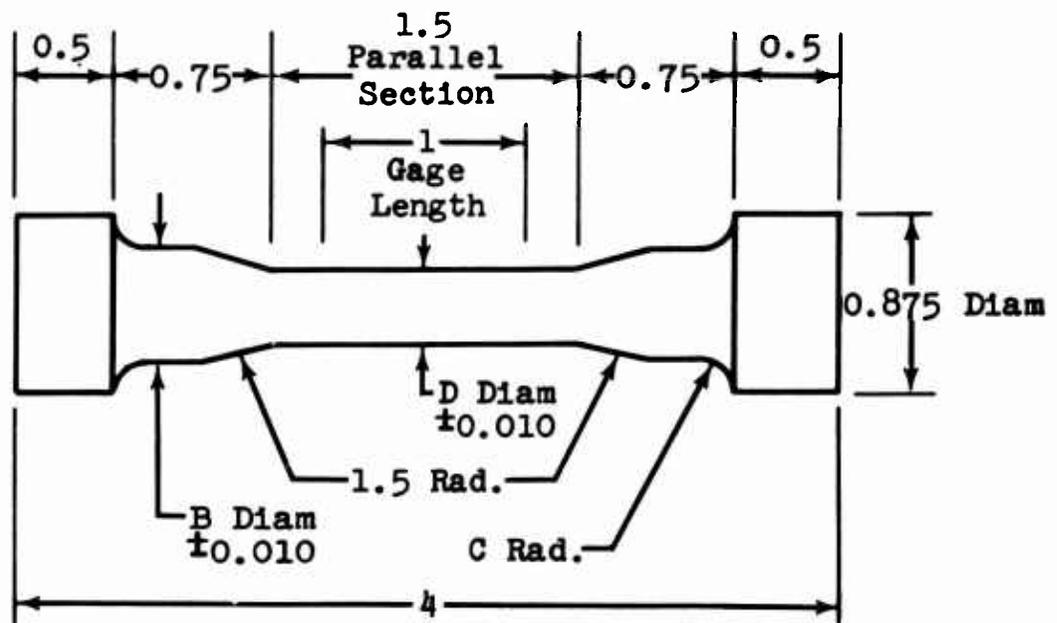
Figure 2-5 Graphite Specimens
