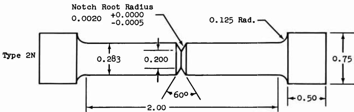
Figure 2-3 Metal Tensile Specimens - Types 1 and 2
