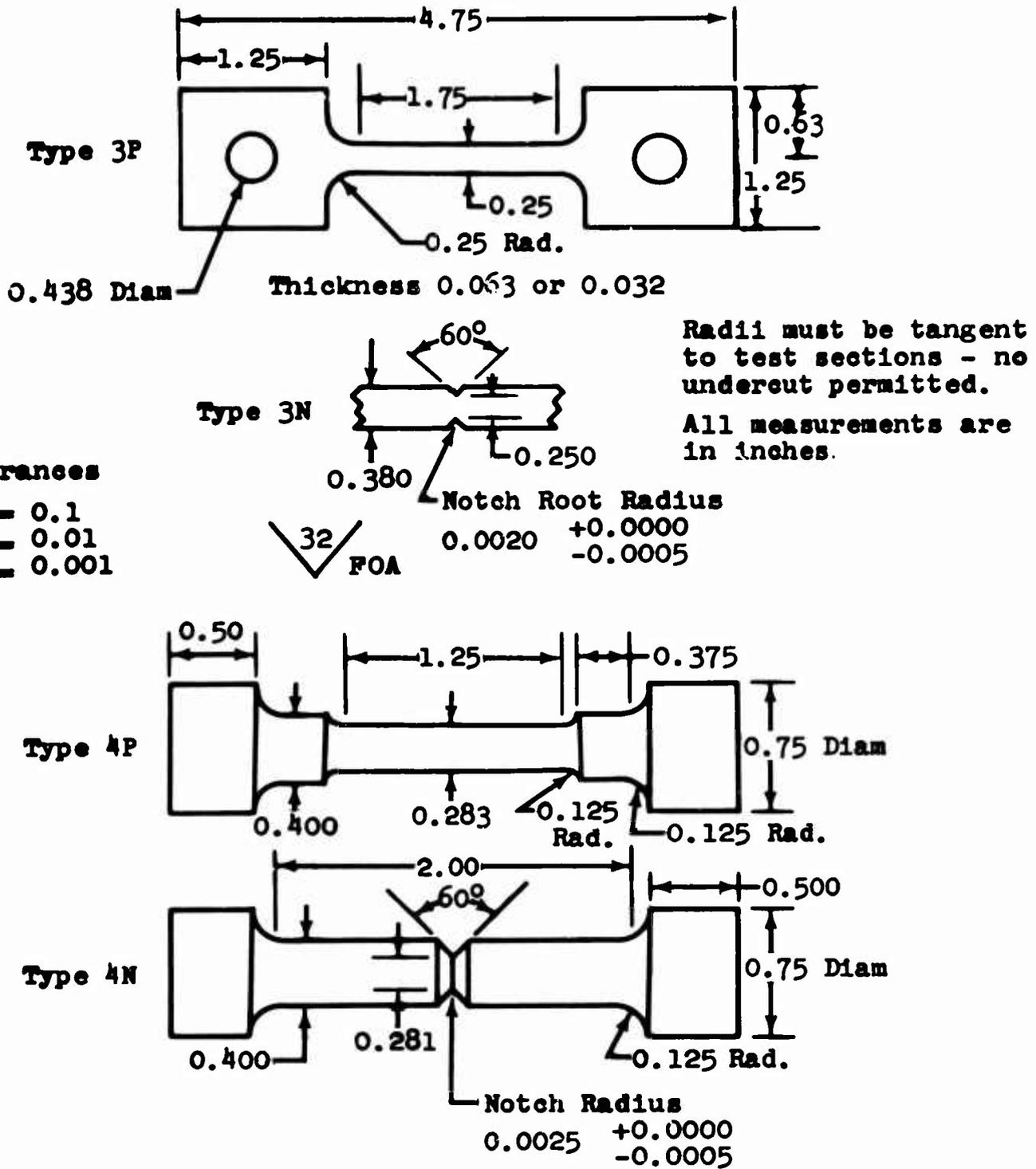
Figure 2-4 Metal Tensile Specimens - Types 3 and 4
