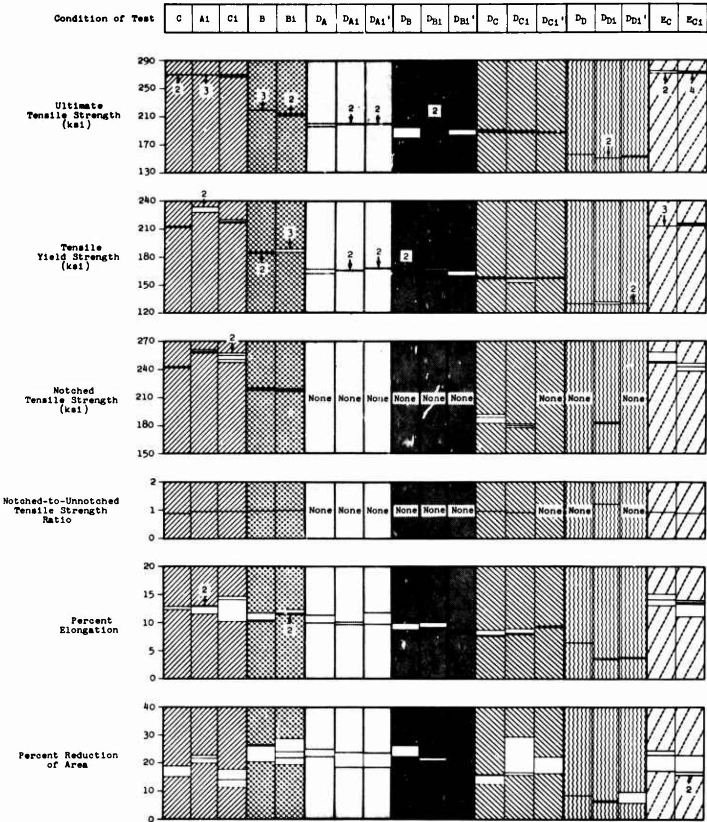
Figure 3-1 Summary of Tensile Test Results: Inconel 718, Type 3
