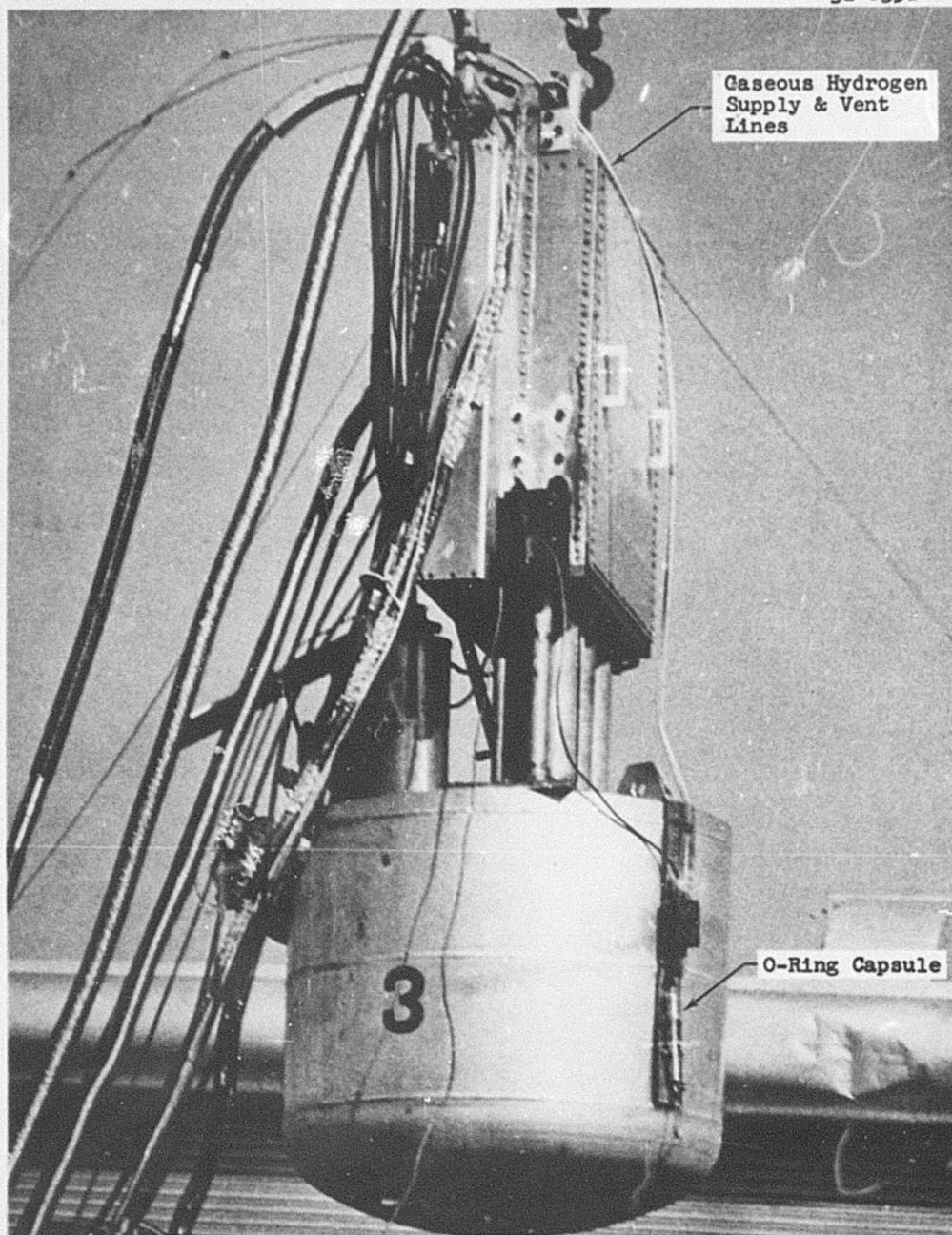
Figure 2-28 O-Ring Capsule Irradiation Configuration - East Dewar
