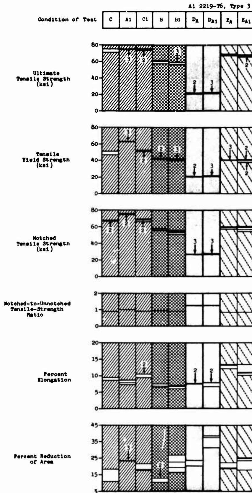
Figure 3-5 Summary of Tensile Test Results: Al 2219-T6, Type 3
