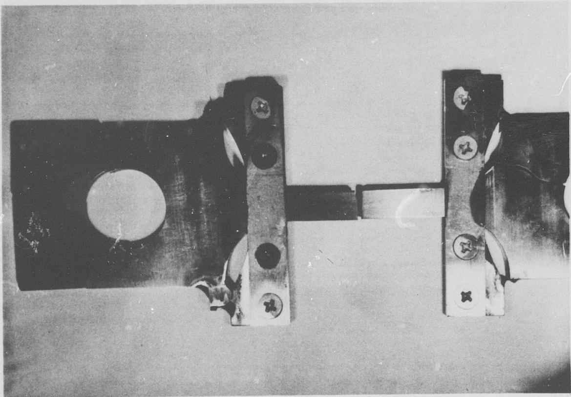
Figure C-138 Stainless Steel 440C, Condition L: Macro-
