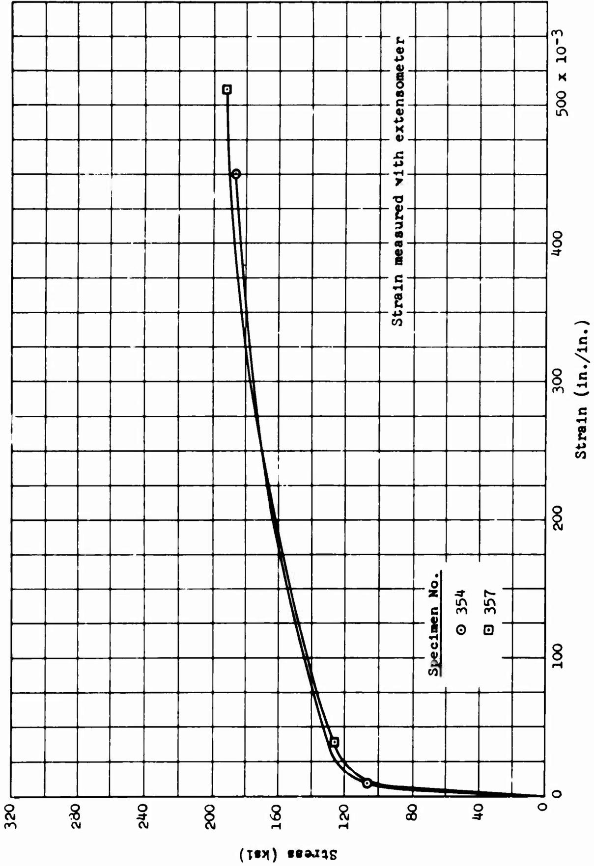
Figure C-183 Hastelloy C, Condition LU: Stress-Strain Curves.
