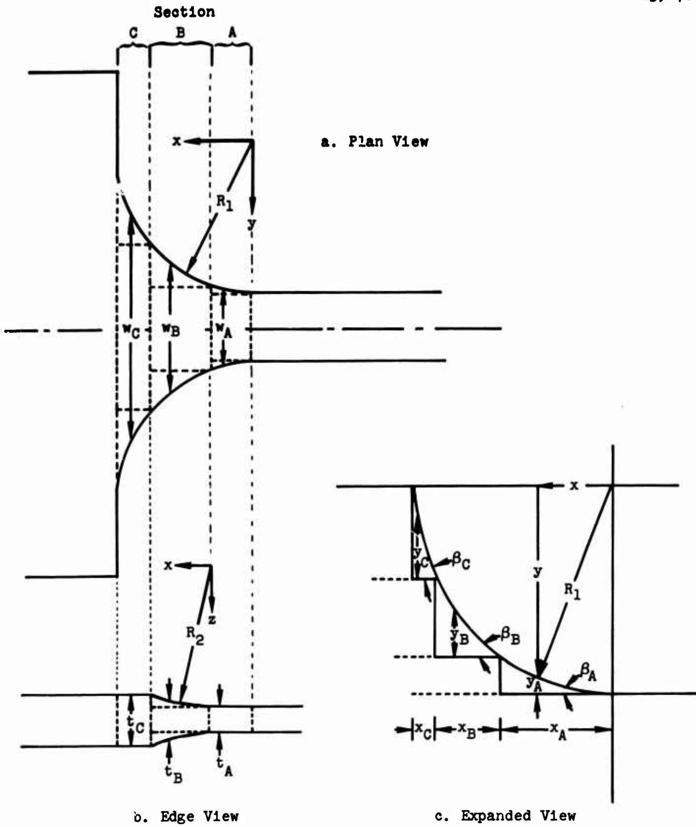
Figure B-2 Geometry of Curved Section
