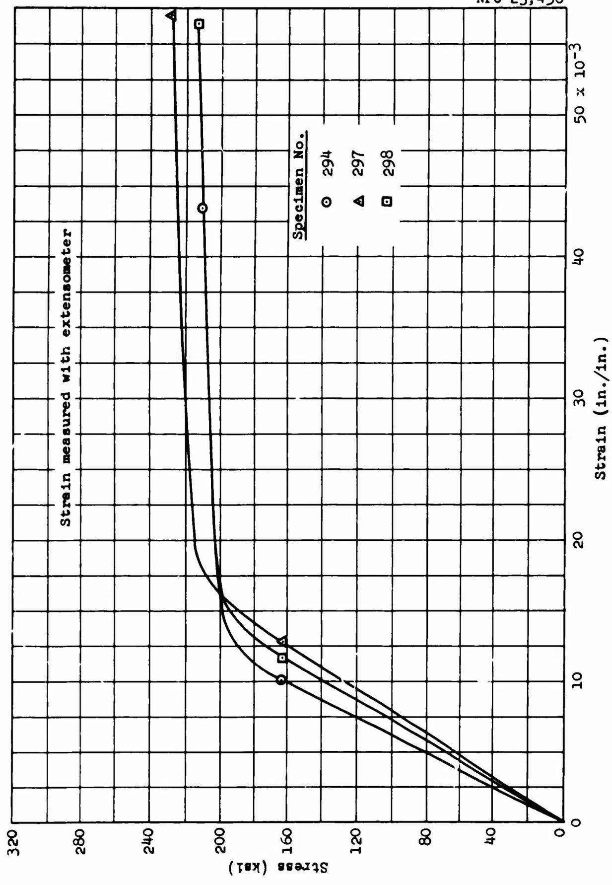
Figure C-211 Titanium A-110-AT, Condition TWU: Stress-Strain Curves
