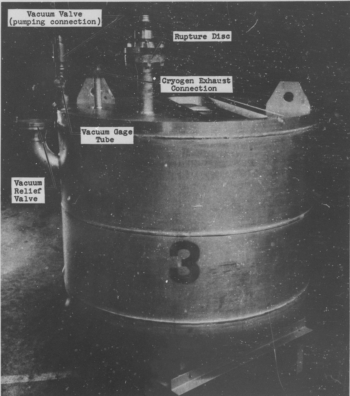
Figure 2-8 Dewar for AGC Cryogenic Materials Test Assembly
