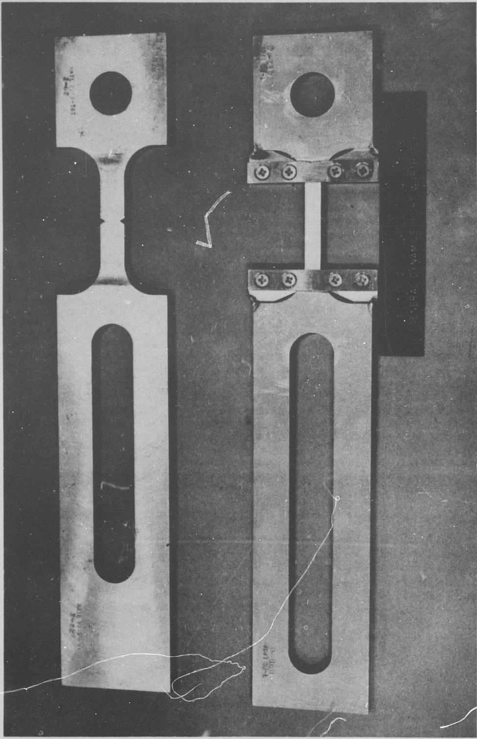
Figure 2-5 Typical AGC Notched and Unnotched Tensile Specimens
