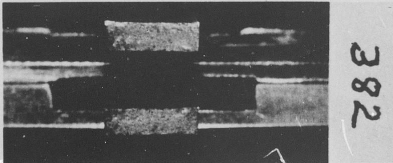
Figure C-158 Inconel X-750, Condition L: Macrograph Showing 3X Magnification of Specimen
