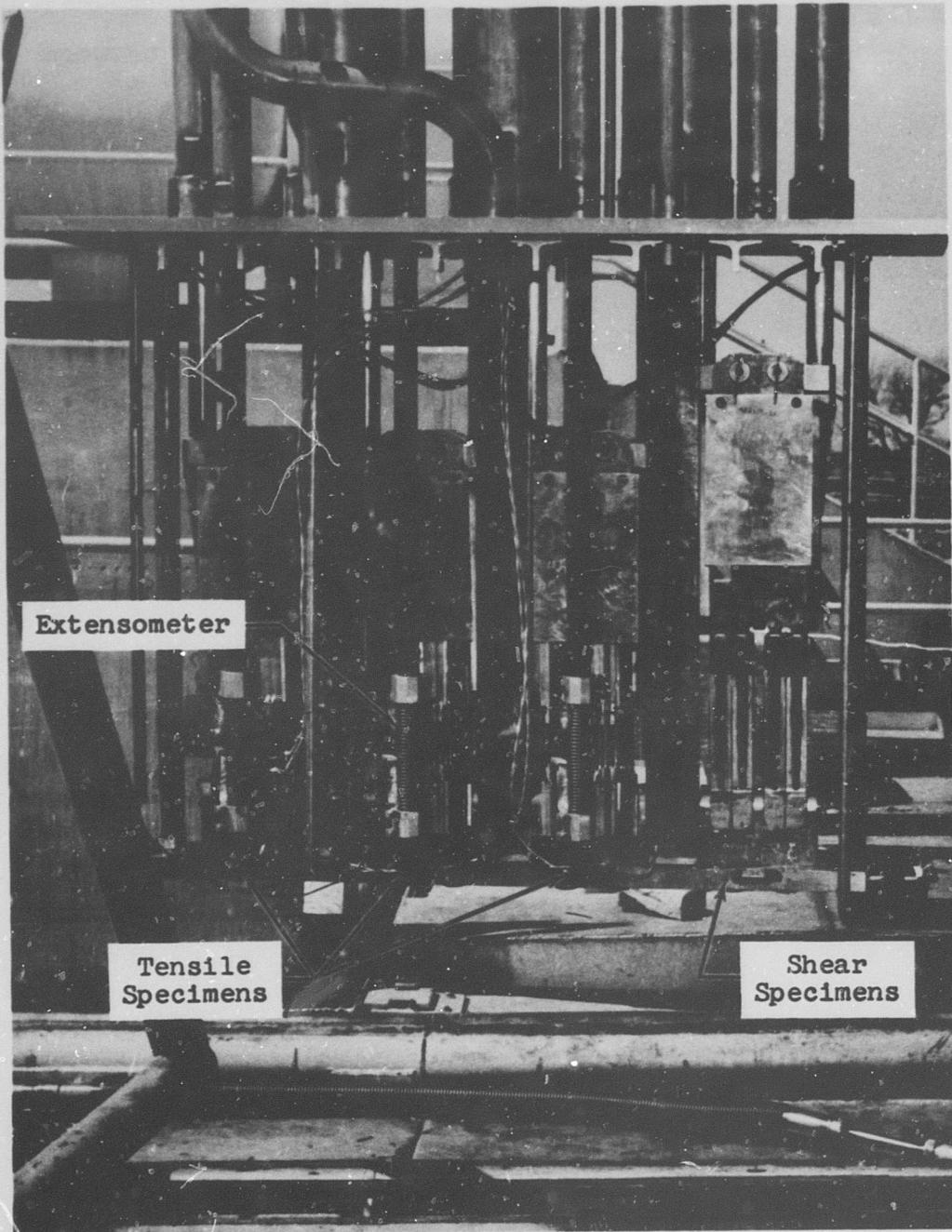
Figure 2-2 Typical Specimen Loading for AGC Cryogenic Materials Test Assembly
