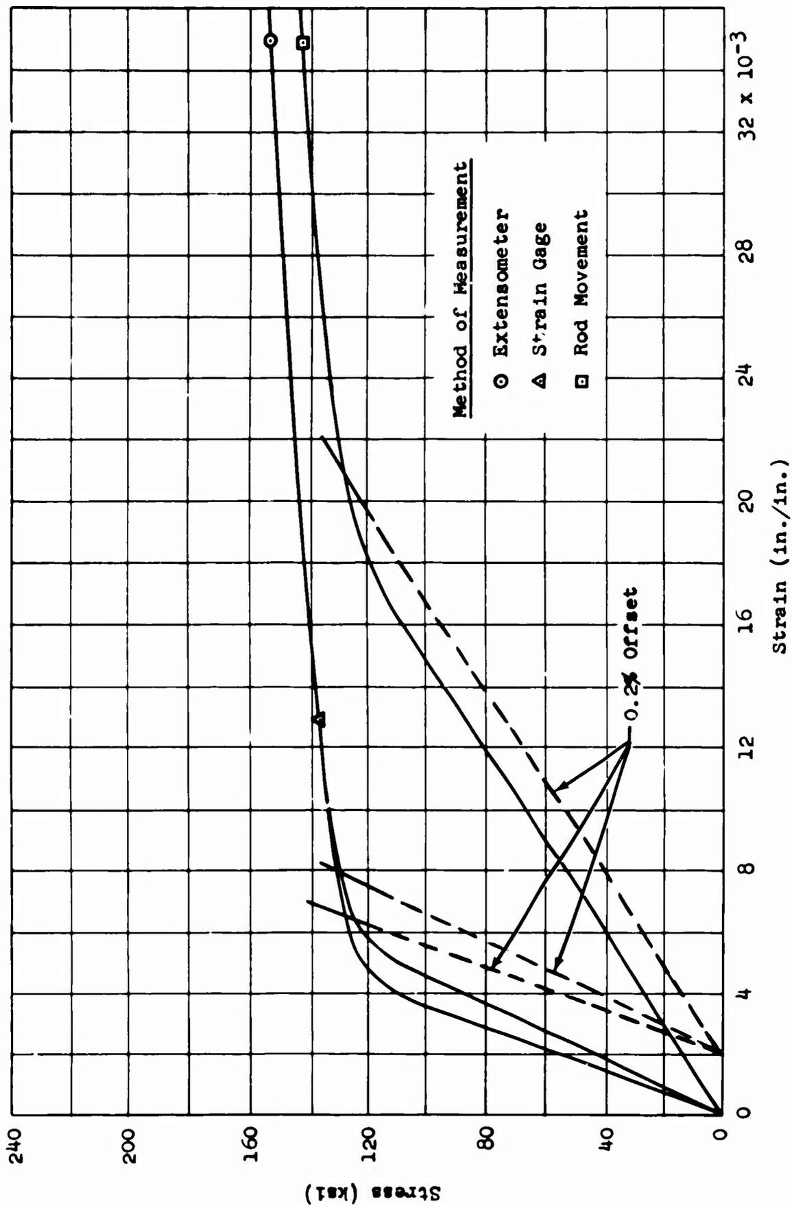
Figure C-142 Stainless Steel A-286, Condition LU: Comparison of Strain-Measurement Methods
