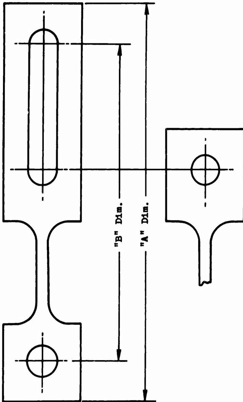
Figure 2--4 Representative Sketch of Specimen Showing Variation in Slot Length
