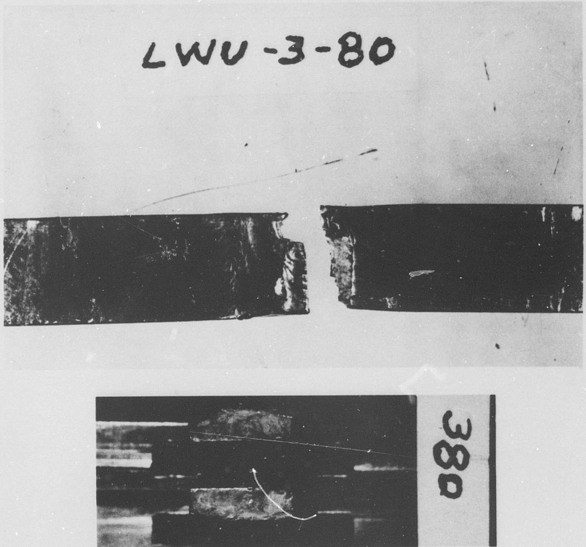
Figure C-31 Aluminum 6061-T6, Condition LW: Macrophotograph Showing 3X Magnification of Specimen
