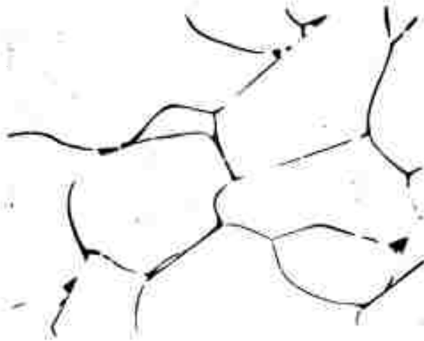
Figure 37. Zr-Hf-B (3/30/67): Sample Quenched from its Melting Point, 3280°C. X400 Diboride Grains in a Metal Matrix (Analyzed Boron Content: 65 Atomic Percent).
