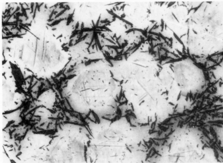
Figure 26. Zr-Hf-B (25/65/10): Arc-Melted Alloy Showing Primary Metal in a Metal-Monoboride Eutectic Matrix. X450
