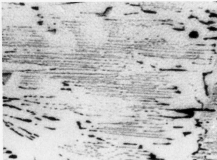
Figure 12. Micrograph of an Arc-Melted Zr-W-B (2/27.5/70.5) Alloy. X2500
