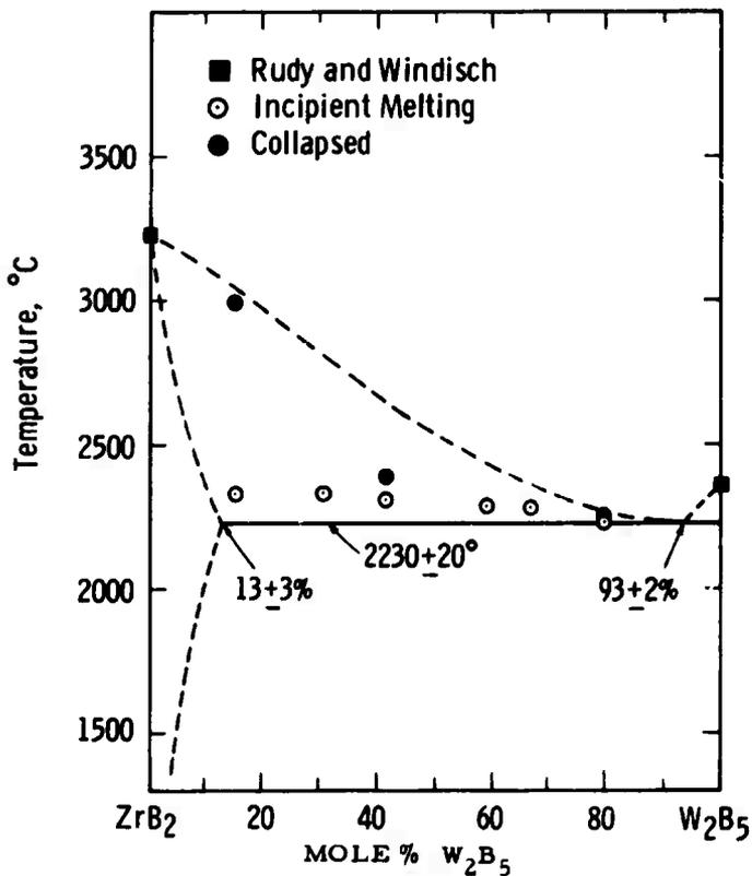
Figure 11. The Phase Diagram for the Pseudobinary System  $ZrB_2$ - $W_2B_5$ .
