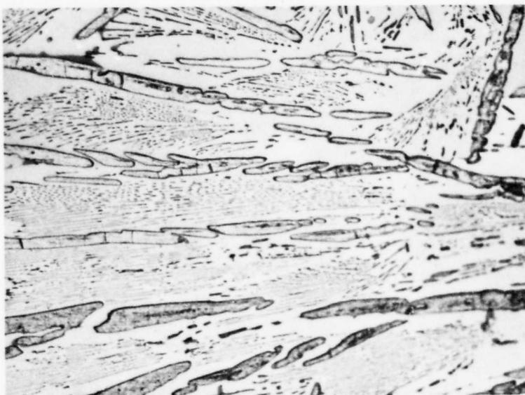
Figure 13. Micrograph of an Arc-Melted Zr-W-B (6/24/70) Alloy. X500
