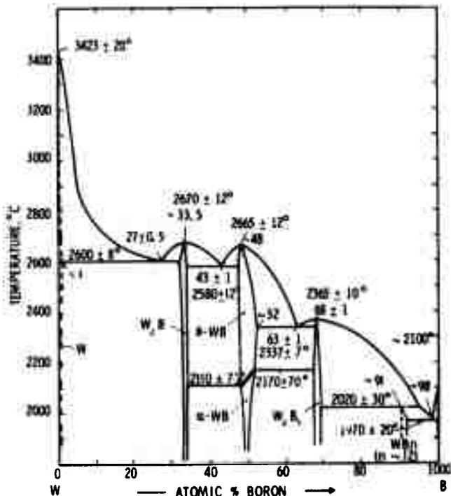
Figure 5. The Constitutional Diagram Tungsten-Boron.
