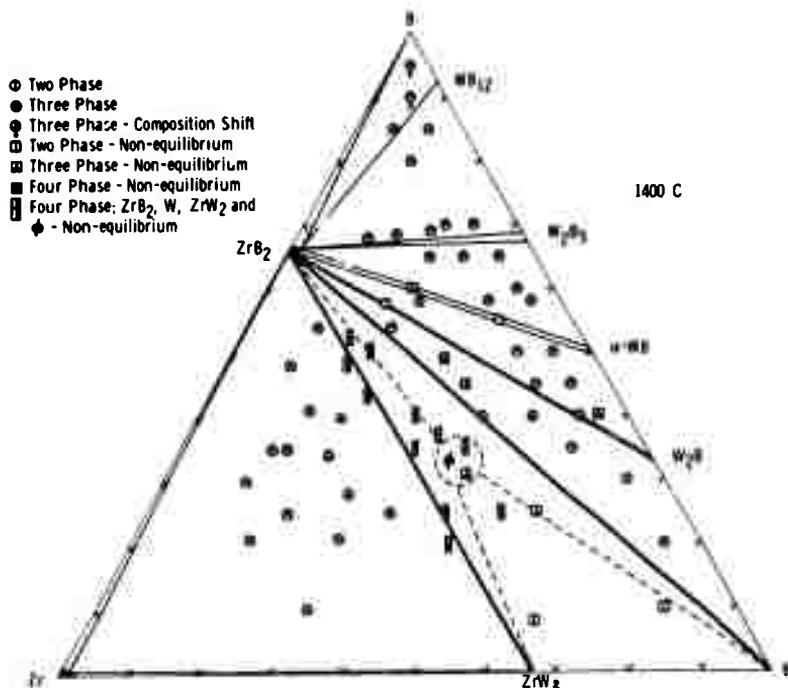
Figure 10. Phase Equilibria of Zr-W-B System at 1400°C, According to X-ray Analysis.
