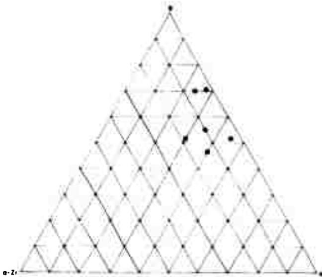
Figure 9. Zr-W-B System: Compositions of Metallographic Samples.
