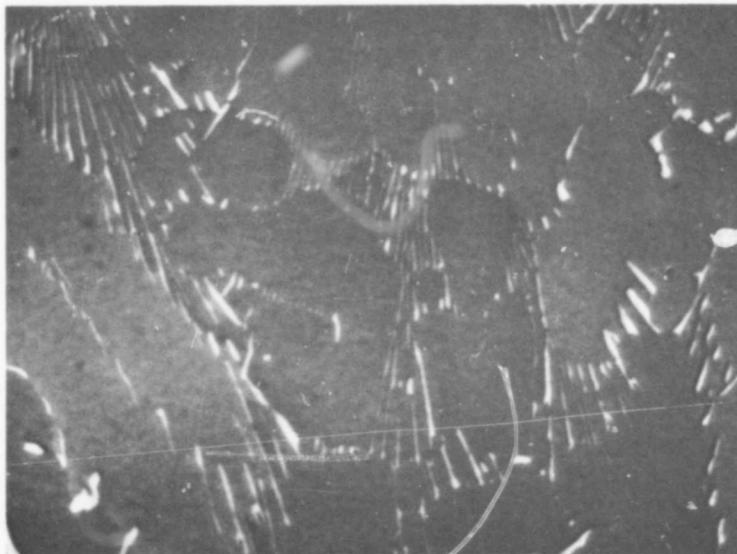
Figure 15. Micrograph of an Arc-Melted Zr-W-B
