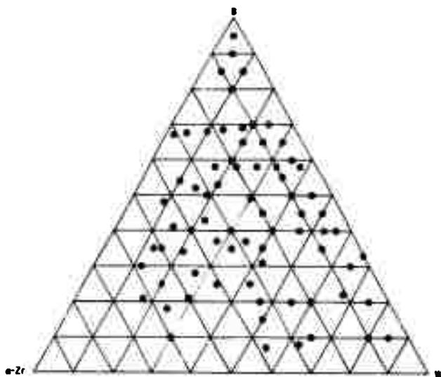
Figure 7. Zr-W-B System: Compositions of Solid State Samples.
