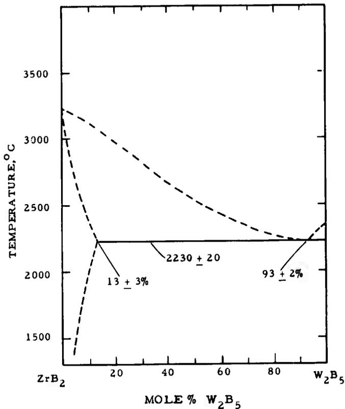
Figure 2. The Pseudobinary System  $ZrB_2$ - $W_2B_5$
