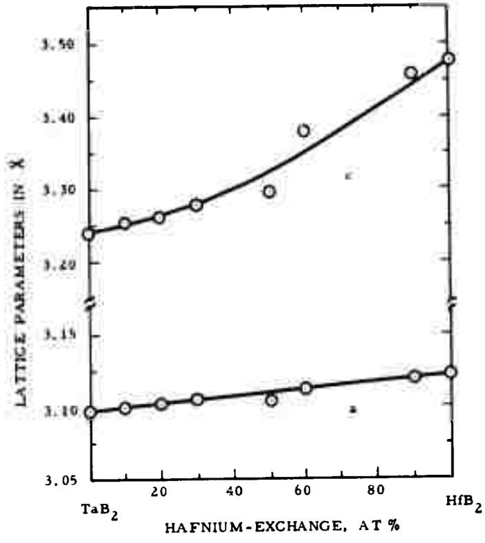
Figure 17. Lattice Parameters of (Ta,Hf)B<sub>2</sub> Solid Solutions.
