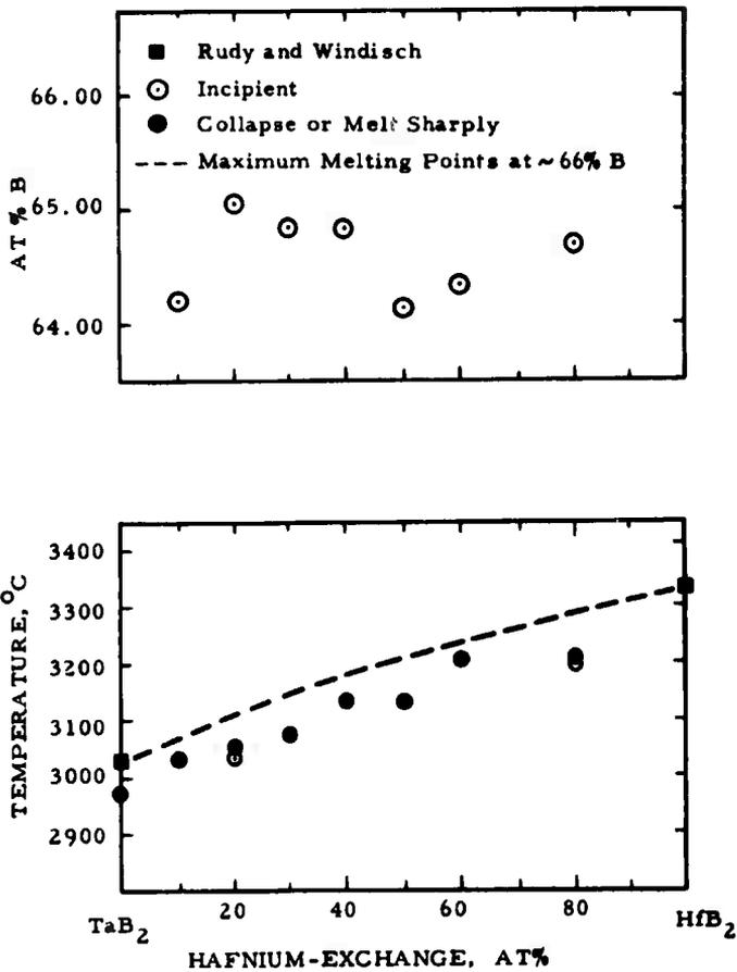
Figure 18. Compositions(Top) and the Melting Temperatures of (Ta, Hf)B<sub>2</sub> Solid Solutions.
