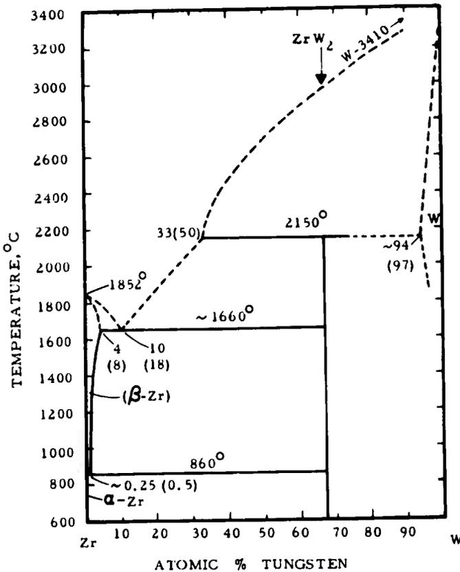
Figure 3. The Constitutional Diagram Zirconium-Tungsten.
