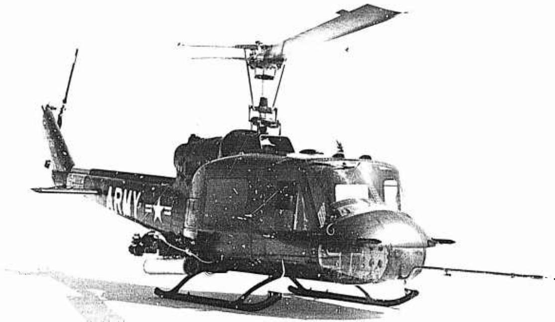
Photo 1 - UH-1B Equipped with XM-21 Armament Subsystem
