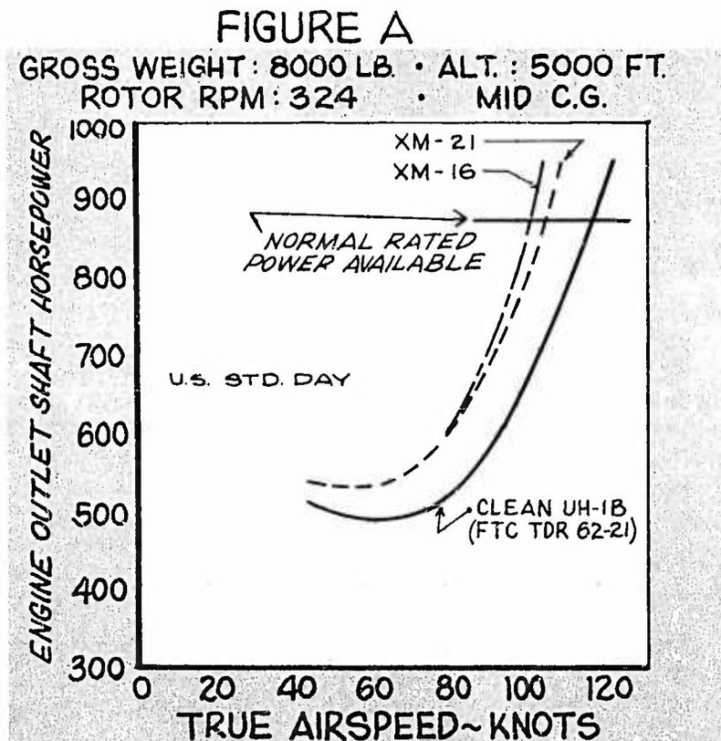
Compared with the performance of a clean UH-1B at the conditions of Figure A, at the airspeed for normal rated power, the installation of the armament subsystems resulted in a 13-knot airspeed loss for the XM-21 and a 16.5-knot airspeed loss for the XM-16.
