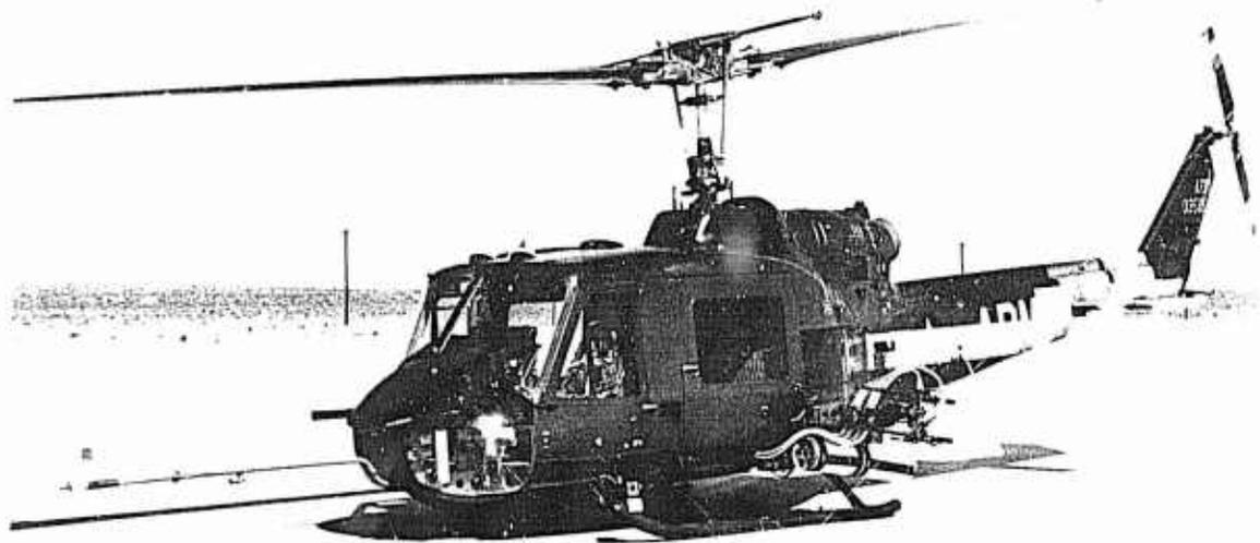
Photo 2 - UH-1B Equipped with XM-16 Armament Subsystem
