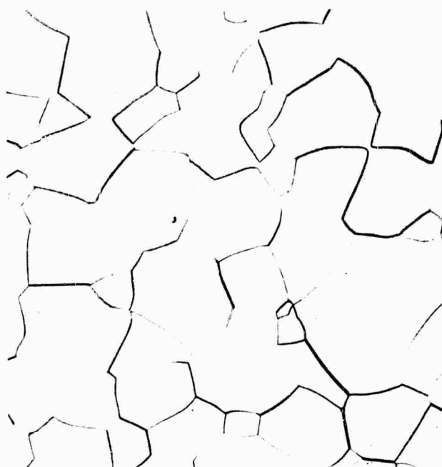
c. Recrystallized High Carbon (35 Ppm C)
