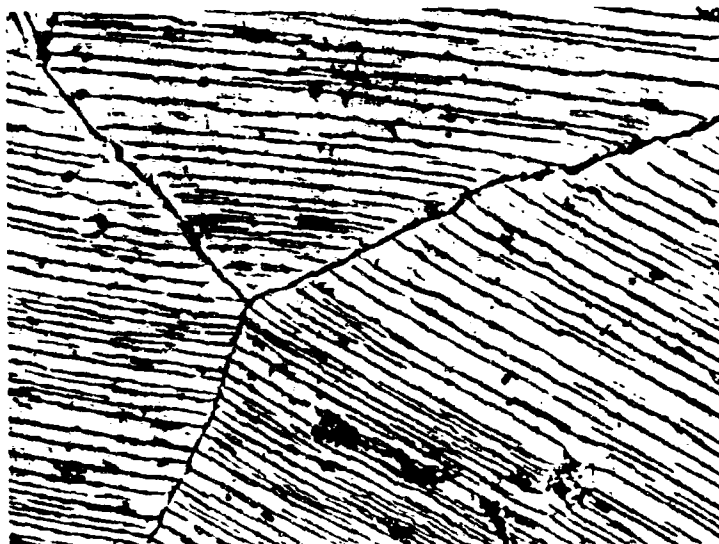
Figure 18. Ta-C (26 At% C), Quenched from 2870°C X750
