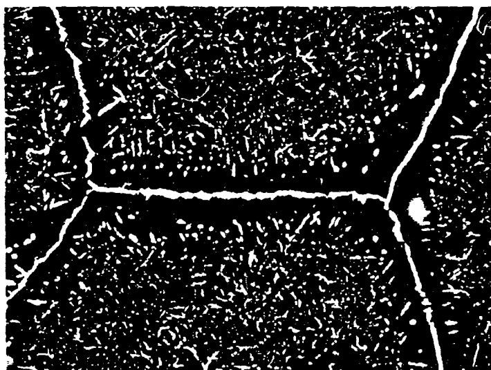
Figure 9. Ta-C (4 At% C), Cooled at Approximately 40^{\circ}C \text{ sec}^{-1} X400 From 2900^{\circ}C .
