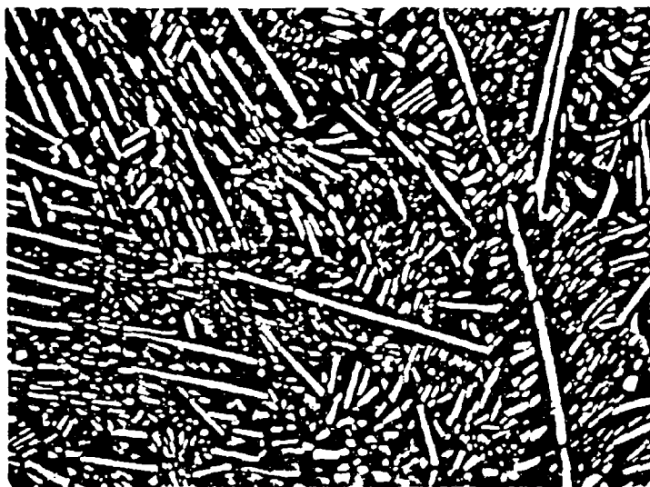
Figure 15. Ta-C (12 At% C), Quenched from 2850°C Ta + Ta 2 C Eutectic
