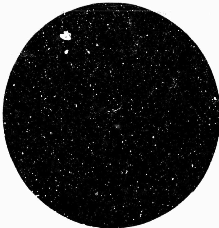
FIGURE 35 COATING DAMAGED BY OPERATION OF THE WINDOW AT 105 MW PEAK AND 52 KW AVERAGE POWER. WINDOW DIAMETER IS 3.14 INCHES.
