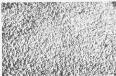
d. 22.5- \mu Aluminum Oxide Grinding Grit
