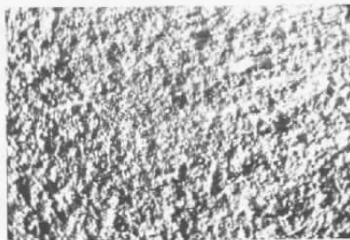
e. 32.0- \mu Aluminum Oxide Grinding Grit
