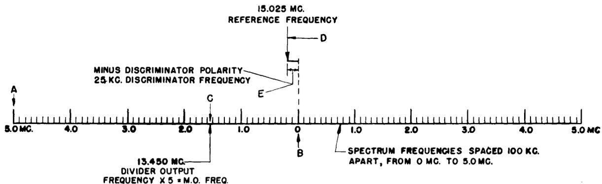
Figure 49.-Relationship between Frequencies in the Monitor for Channel Number 345.
