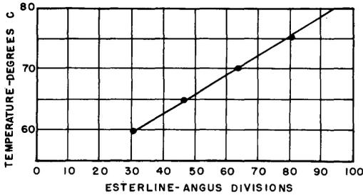
Figure 86.-Calibration for Thermistor Bridge
