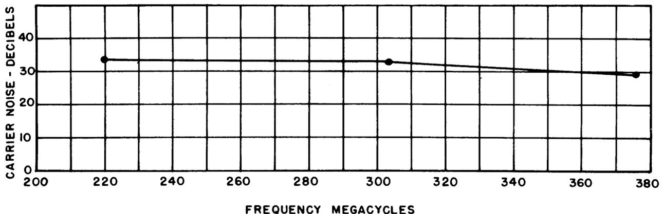
Figure 154.-Transmitter Noise Modulation of AN/ARC-19 (XN-1), Serial Number 4, at Room Ambient Conditions; Primary Supply 26.5 Volts.
