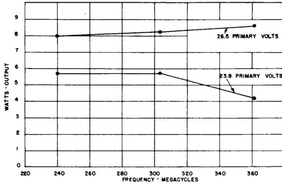
Figure 145.—Transmitter power output (at  $-50^{\circ}\text{C}$  ambient temperature) of AN/ARC-19 (XN-1), serial number 4, with 50-ohm resistive load.
