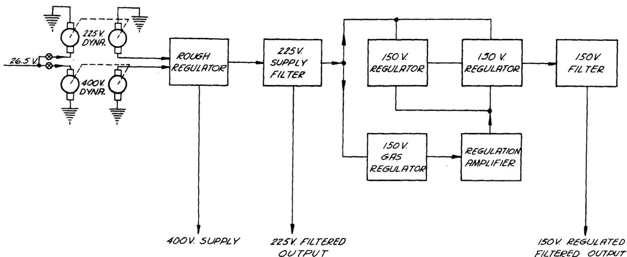
Figure 32.-Block Diagram of Power Supply and Filters.
