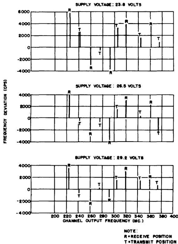
Figure 163.-Channel frequency deviations at  $-50^{\circ}\text{C}$  ambient temperature for AN/ARC-19 (XN-1), serial number 3.
