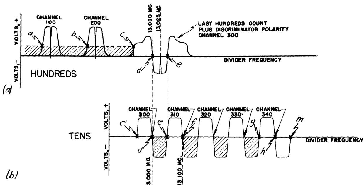
Figure 45.-Signals at Trigger Tube Grid for Hundreds and Tens Count.
