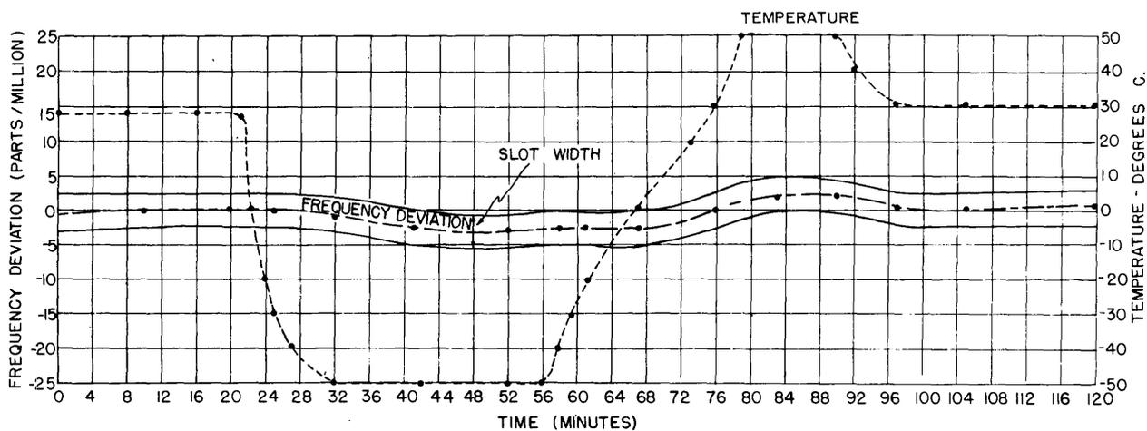
Figure 80.-Frequency deviation vs time during a cyclic temperature run at channel 990, on monitor number 2, with master oscillator at room temperature.
