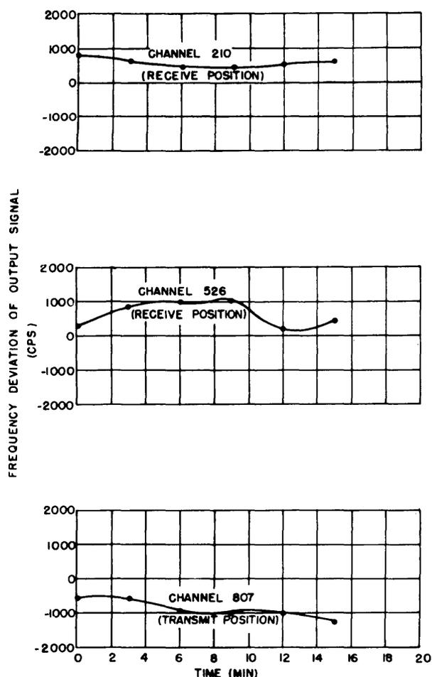
Figure 162.—Frequency stability at  $+50^{\circ}$  C ambient temperature for AN/ARC-19 (XN-1), serial number 3; primary supply is 26.5 volts.
