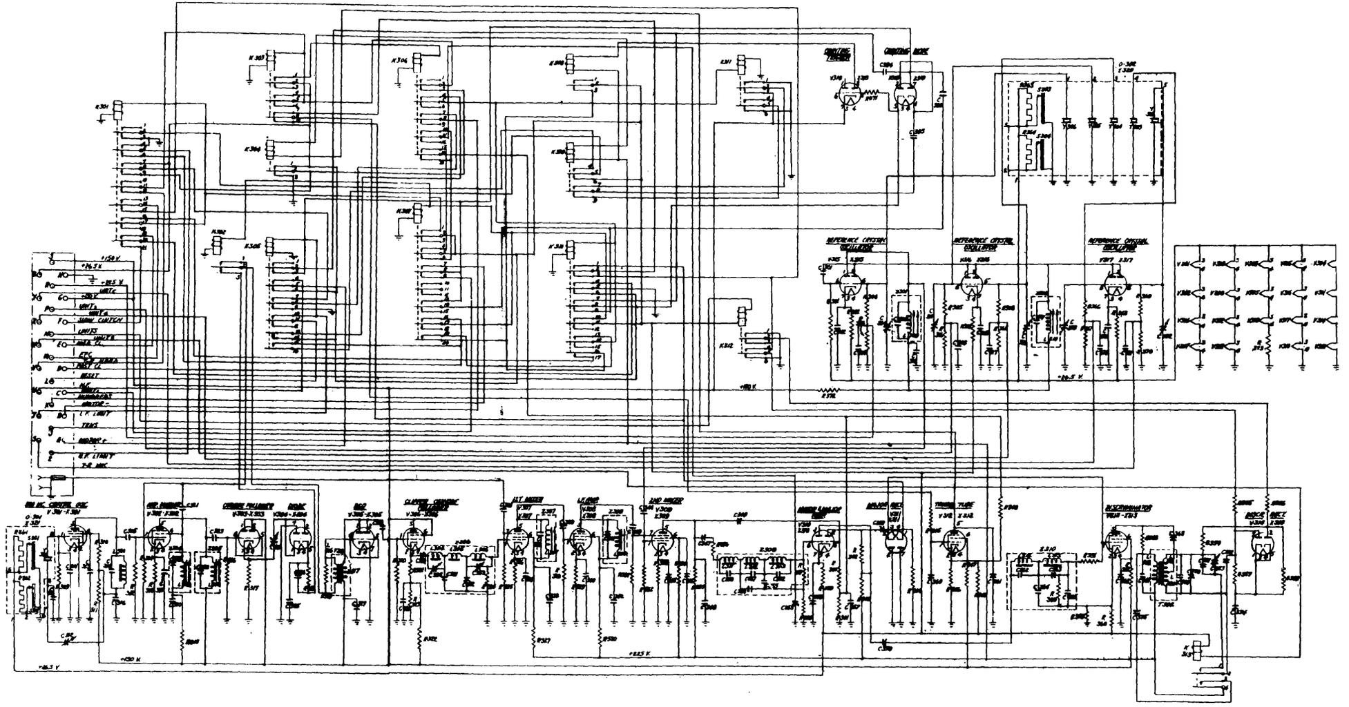
Figure 167.-Schematic Diagram of Electronic Counting Type Monitor
