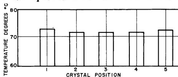
Figure 91.-Oven Temperature variation with change in crystal position for five-unit, model 2 oven, serial number 8, at room ambient conditions.
