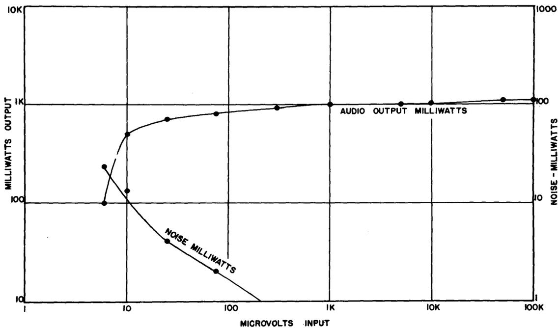
Figure 129.—Receiver AVC characteristics of AN/ARC-19 (XN-1), serial number 4, at -50°C ambient temperature with primary supply 26.5 volts. Frequency is 361.4 Mc; input is 30 percent modulated at 1,000 cps.
