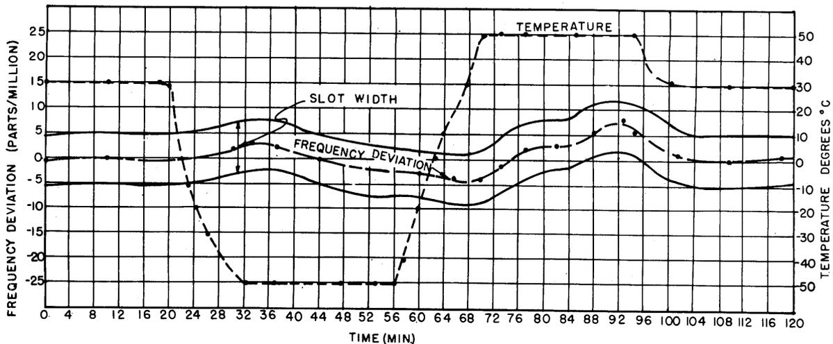
Figure 84.-Frequency deviation vs time during a cyclic temperature run at channel 100, on monitor number 5, with master oscillator at room temperature.
