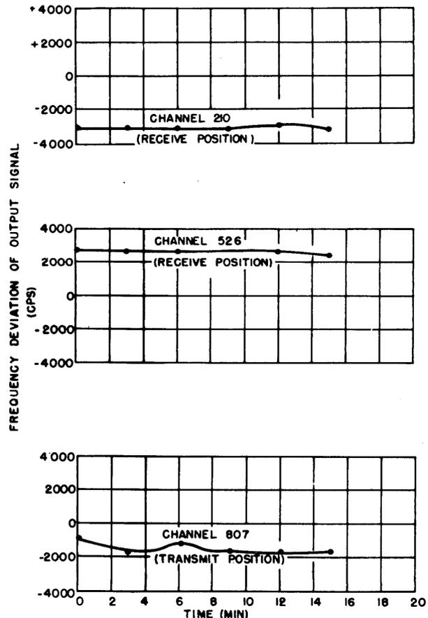
Figure 161.—Frequency stability of AN/ARC-19 (XN-1), serial number 3, at  $-50^{\circ}\text{C}$  ambient temperature; primary supply is 26.5 volts.
