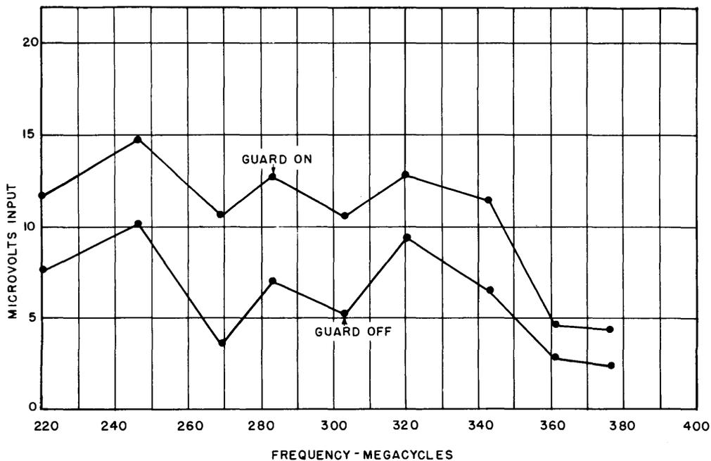
Figure 119.-Receiver main channel sensitivity of AN/ARC-19 (XN-1), serial number 4, at room ambient conditions; primary supply 29.2 volts and squelch disabled.
