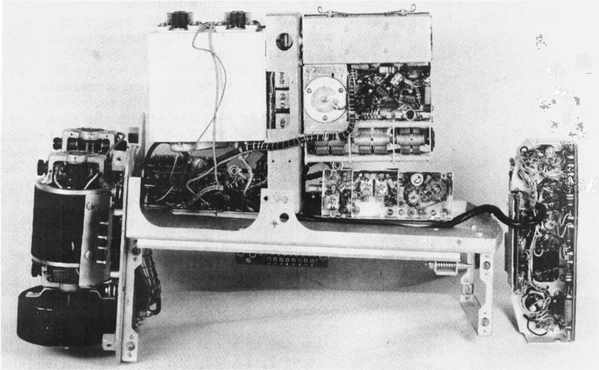
Figure 23.-Bottom View of R-F Assembly, Guard Channel Receiver, and Modulator Unit.
