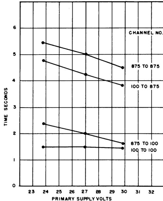
Figure 156.-Channel selection time of AN/ARC-19 (XN-1), serial number 3, at room ambient conditions.
