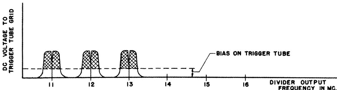
Figure 40.-Signals at Trigger Tube Grid.
