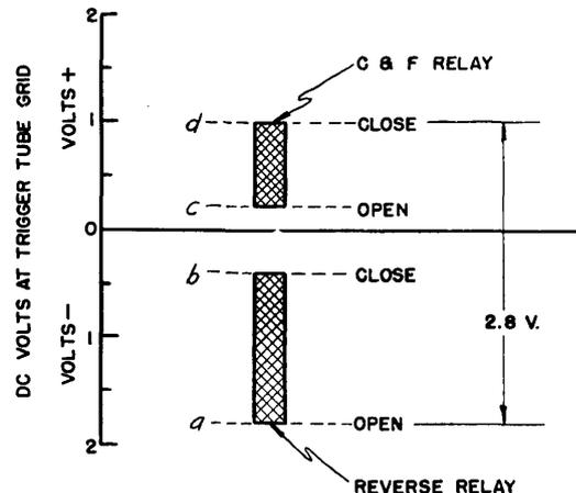
Figure 64.-Reverse C and F Relay Adjustment
