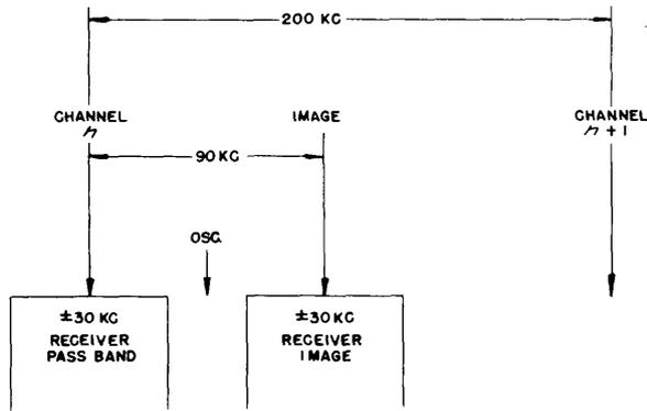
Figure 1.-Frequency Allocation for Receiver with 45-kc I-F
