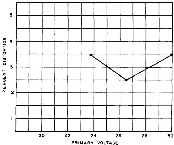
Figure 138.-Receiver audio distortion vs primary supply voltage for AN/ARC-19 (XN-1), serial number 4, at room ambient conditions; input modulated 30 percent at 1,000 cps.
