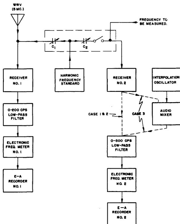
Figure 65.-Block Diagram of Frequency Measuring Setup
