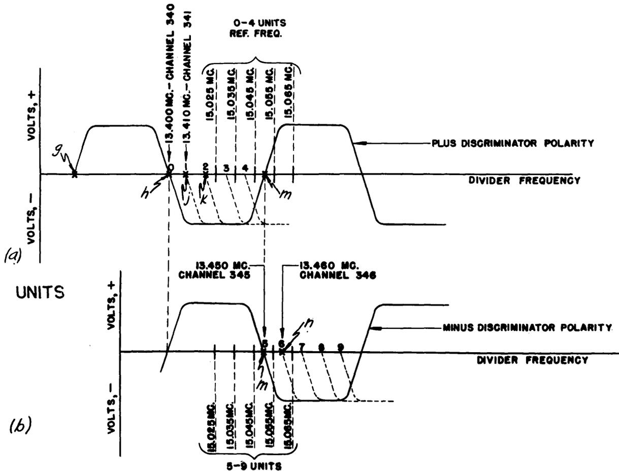
Figure 47.-Signal at Trigger Tube Grid for Units Selection.
