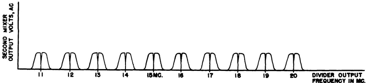
Figure 39.-Second Mixer Audio Output Response vs Divider output Frequency.
