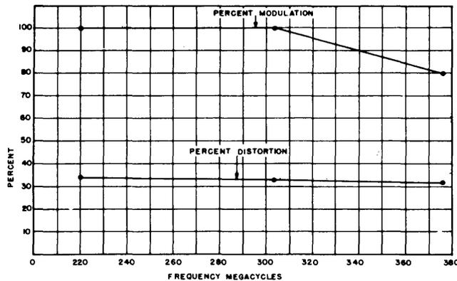
Figure 152.-Transmitter modulation characteristics and distortion with tone operation of AN/ARC-19 (XN-1), serial number 4, at room ambient conditions; primary supply 26.5 volts.
