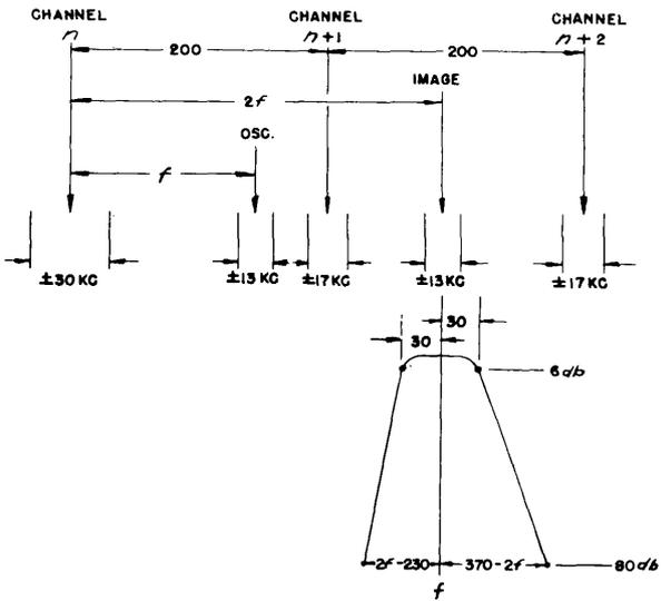
Figure 2.-Frequency Allocation for Receiver with 143-kc I-F
