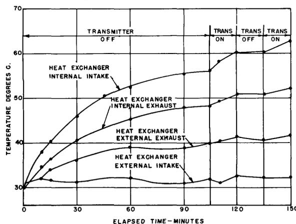
Figure 100.—Heat exchanger temperatures for AN/ARC-19 (XN-1) serial number 2, at room ambient conditions with primary supply 26.5 volts and transmitter cycled after stabilization.
