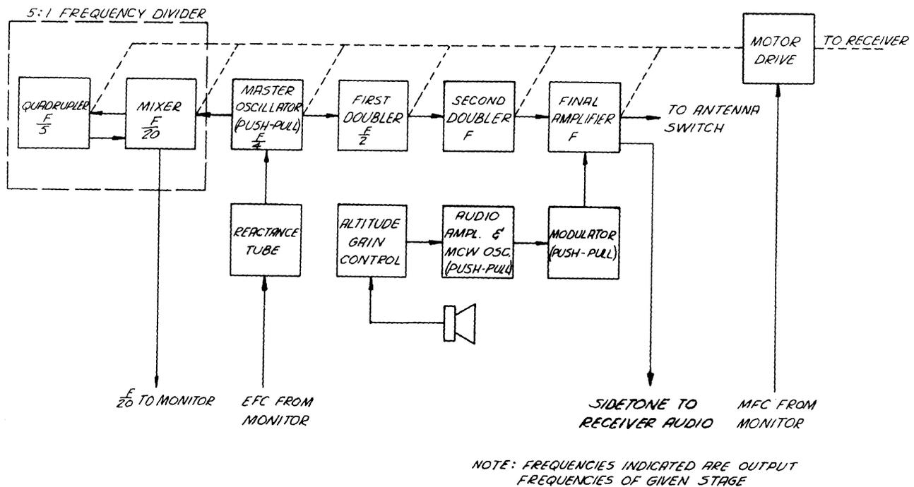
Figure 26.—Transmitter Block Diagram.
