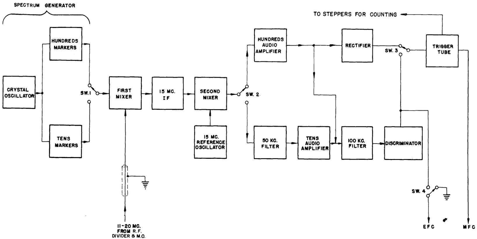
Figure 41.-Simplified Block Diagram of Monitor Unit for Tens Count
