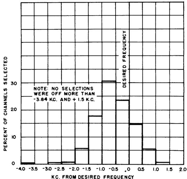
Figure 157.-Distribution of error in frequency for 676 channel selections of AN/ARC-19 (XN-1), serial number 3 at room ambient conditions; primary supply 26.5 volts.
