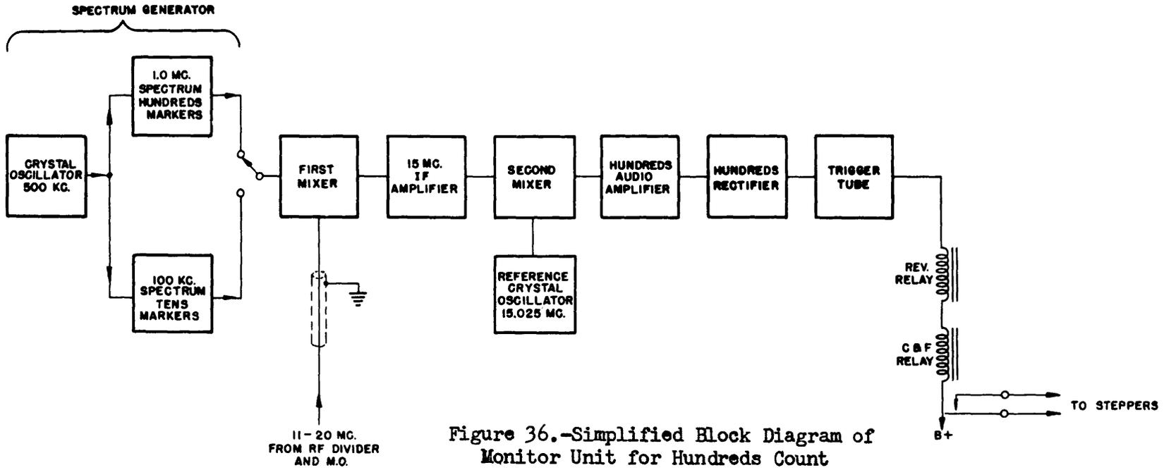
Figure 36.-Simplified Block Diagram of Monitor Unit for Hundreds Count
