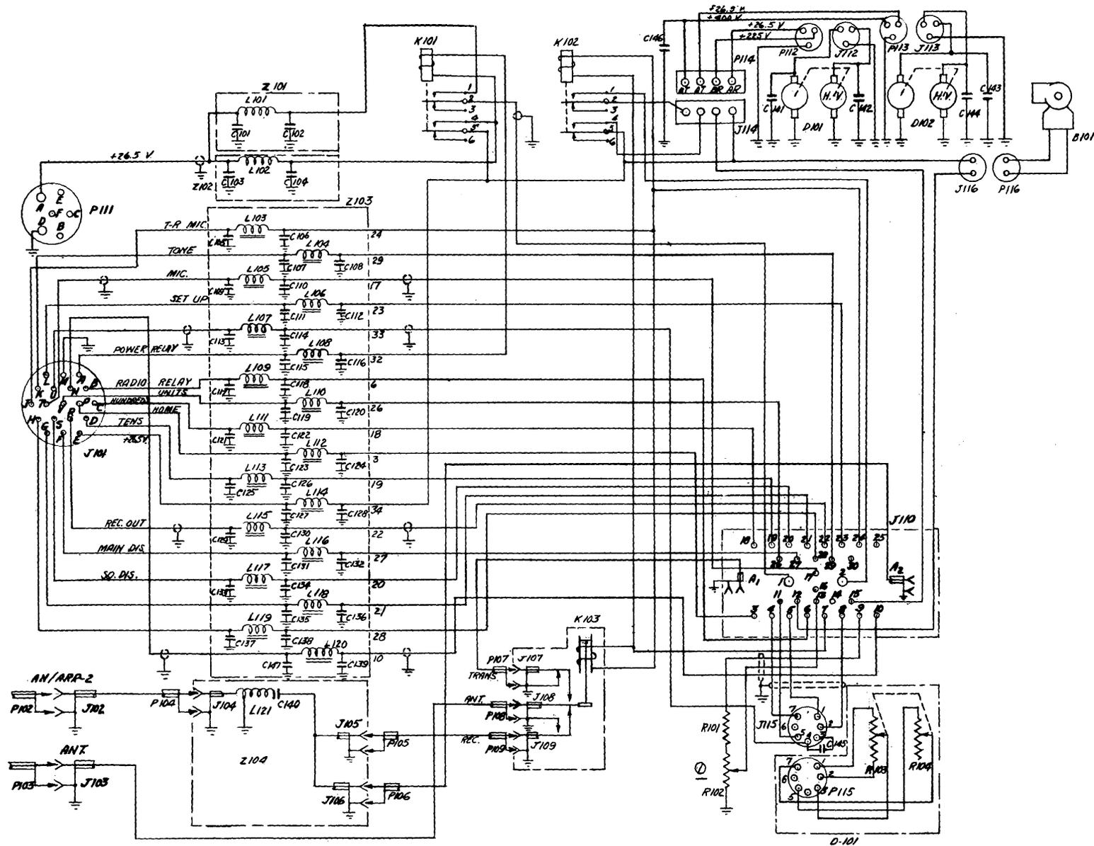
Figure 33.-Schematic Diagram of Head Assembly.
