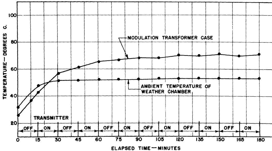
Figure 110.-Equipment Warm-up of AN/ARC-19 (XN-1), serial number 2 at High Ambient Temperature; Primary Supply 26.5 Volts
