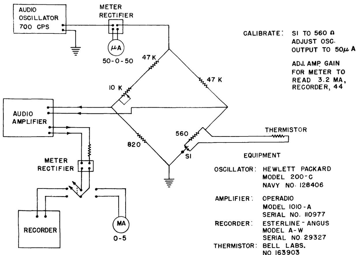
Figure 85.-Thermistor Bridge Circuit for Crystal Oven Internal Temperature Measurements
