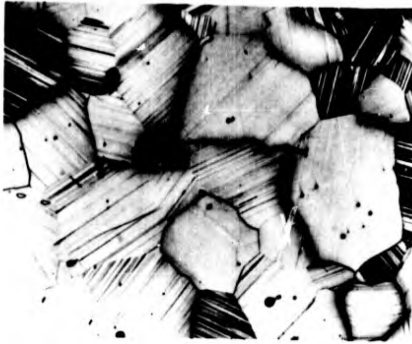
Figure 29. Mo-B (66 At% B), Cooled with \sim 40^\circ\text{C} per Second X200 from 2350^\circ\text{C} .
