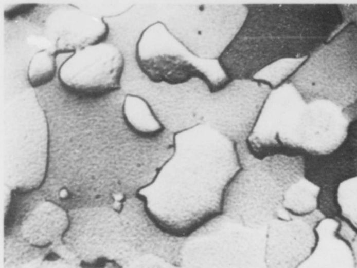
Figure 49. W-B (27.3 At% B), Rapidly Cooled from 2570°C. X2500 Sinterstructure W-W 2 B
