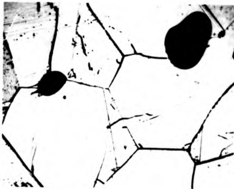
Figure 23. Mo-B (52 At% B), Quenched from 2400°C. X500 \beta -MoB with Pores (Black)
