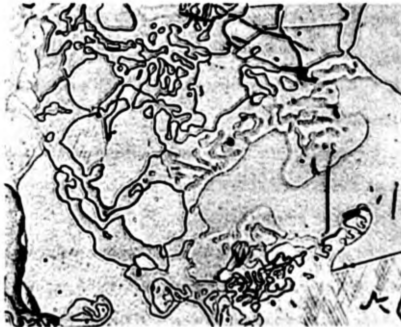
Figure 56. W-B (43 At% B), Cooled with \sim 60^\circ\text{C} per Second from 2590^\circ\text{C} .
