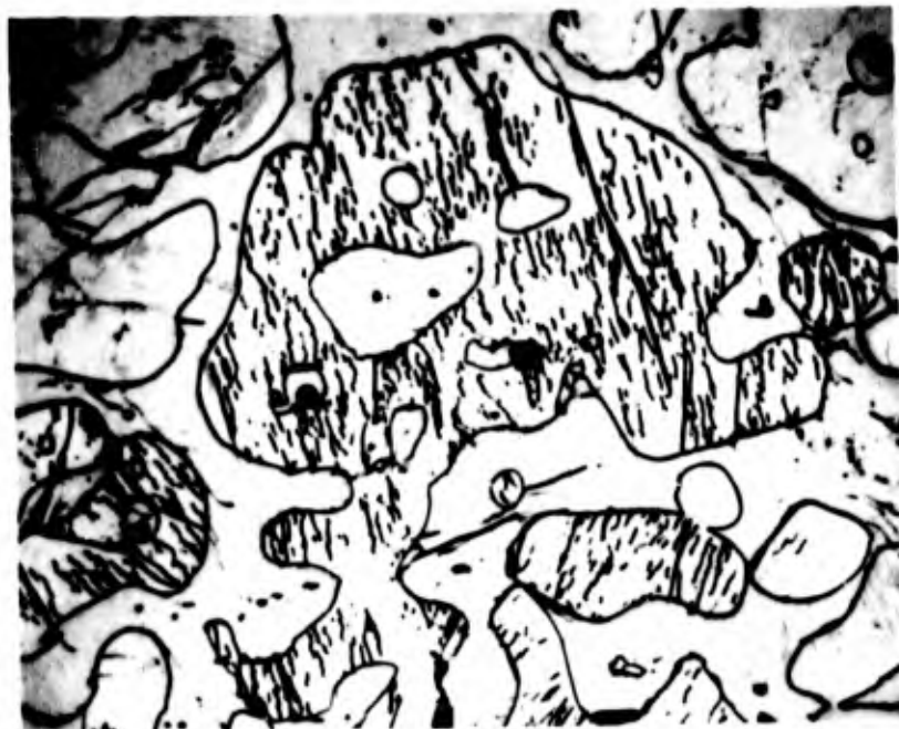
Figure 19. Mo-B (40 At% B), Cooled with \sim 80^\circ\text{C} per Second X500 from 2300^\circ\text{C} .
