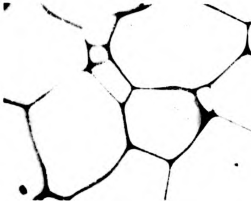
Figure 42. W-B (2 At% B), Quenched ( \sim 90^{\circ}\text{C}\cdot\text{sec}^{-1} ) from X1000 3270°C.
