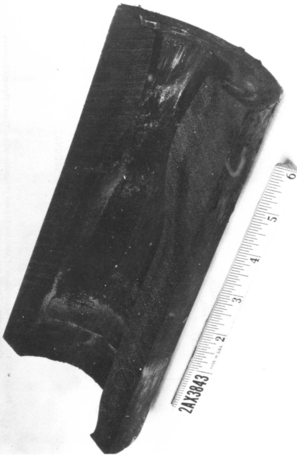
Figure 19. Ablative Phenolic-Graphite Thrust Chamber After Exposure to OF_2 - B_2H_6 Exhaust
