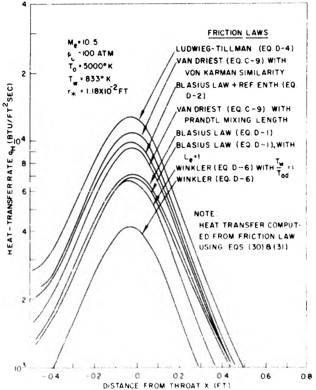
FIG 22 EFFECT OF FRICTION LAW ON CONVECTIVE THROAT HEATING
