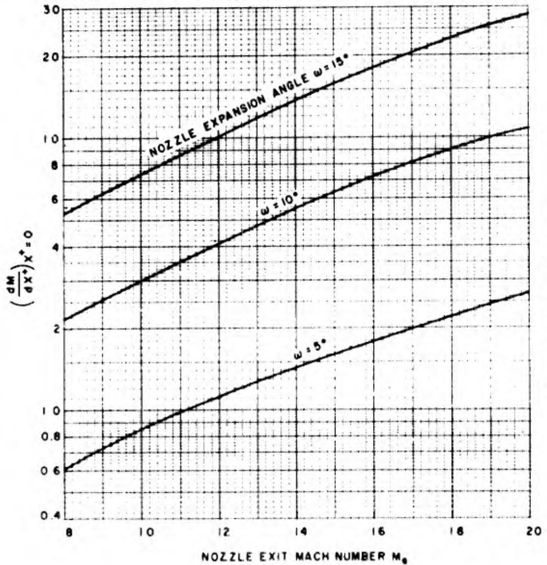
FIG 13 FOELSCH NOZZLE, DIMENSIONLESS THROAT MACH NUMBER GRADIENT
