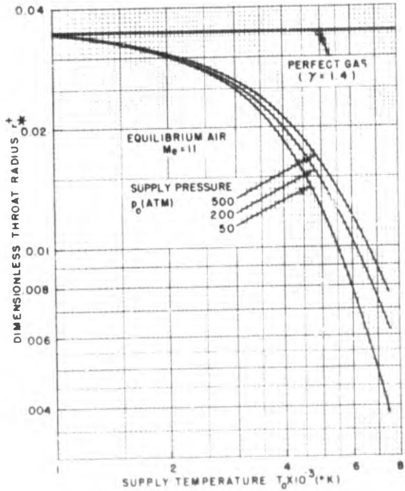
FIG 10 EFFECT OF SUPPLY CONDITIONS ON THROAT SIZE OF MACH 11 NOZZLE
