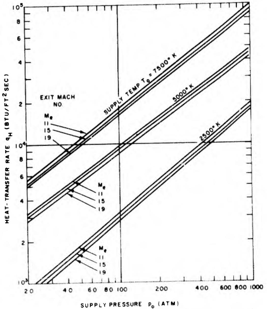
FIG 24 PEAK NOZZLE THROAT CONVECTIVE HEAT-TRANSFER RATE
