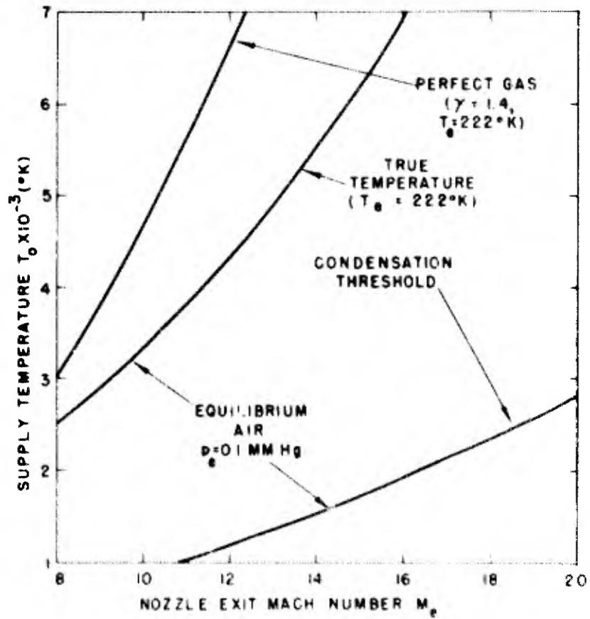
FIG 8 COMPARISON OF SUPPLY TEMPERATURE REQUIREMENTS
