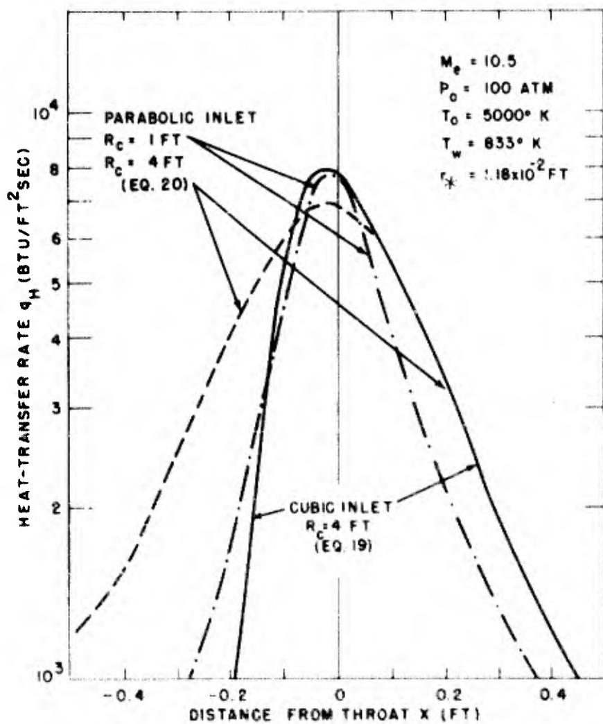
FIG 21 EFFECT OF NOZZLE INLET GEOMETRY ON CONVECTIVE HEAT-TRANSFER RATE
