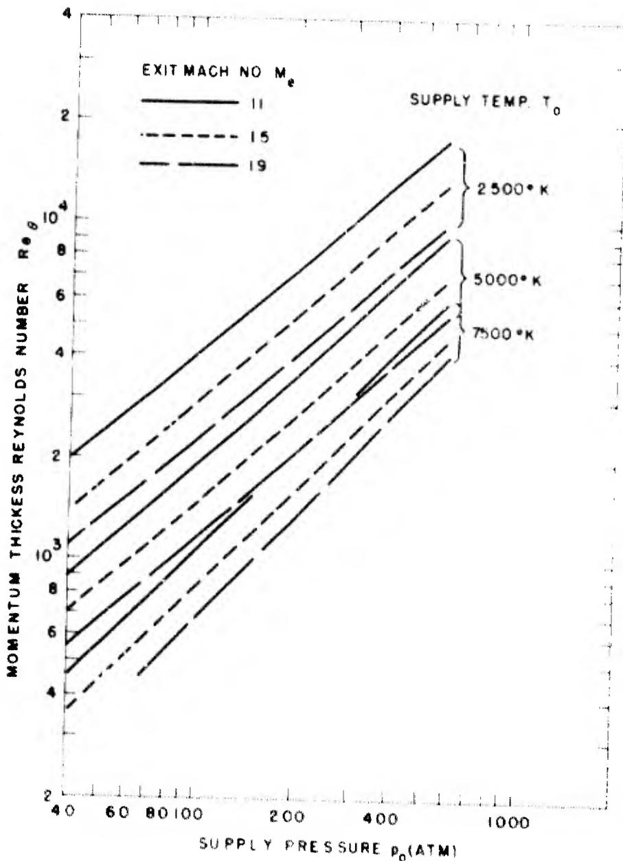
FIG 26 THROAT VALUE OF BOUNDARY-LAYER MOMENTUM THICKNESS REYNOLDS NUMBER
