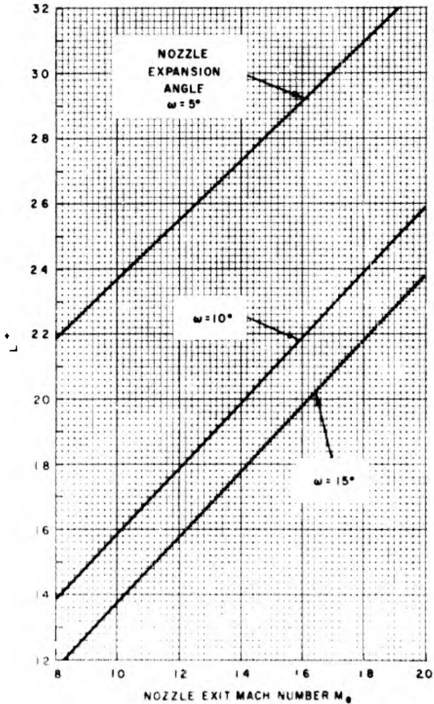
FIG 14 FOELSCH NOZZLE, DIMENSIONLESS THROAT-EXIT LENGTH
