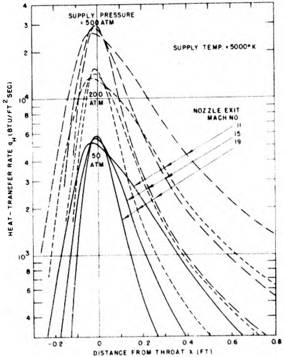
FIG. 23 VARIATION OF HEAT-TRANSFER RATE IN THE THROAT REGION FOR A FAMILY OF NOZZLES
