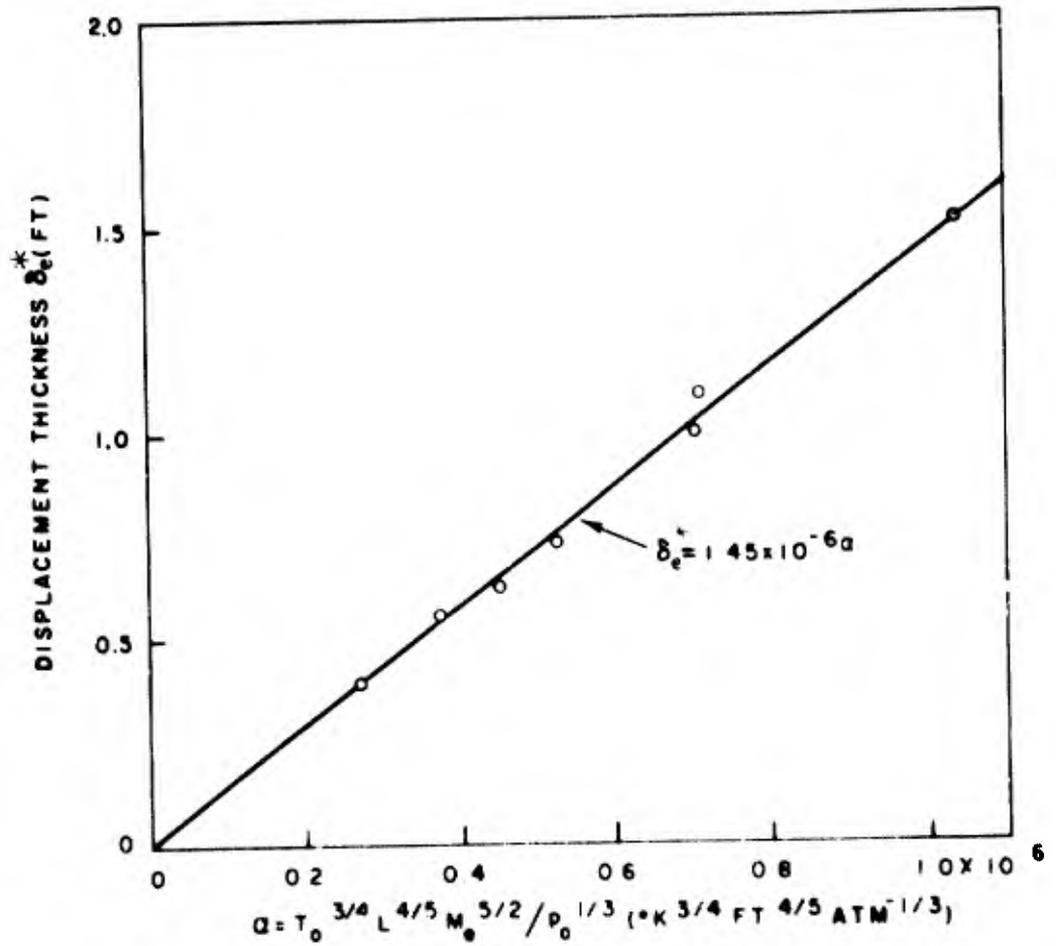
FIG. 28 CORRELATION OF NOZZLE EXIT BOUNDARY-LAYER DISPLACEMENT THICKNESS
