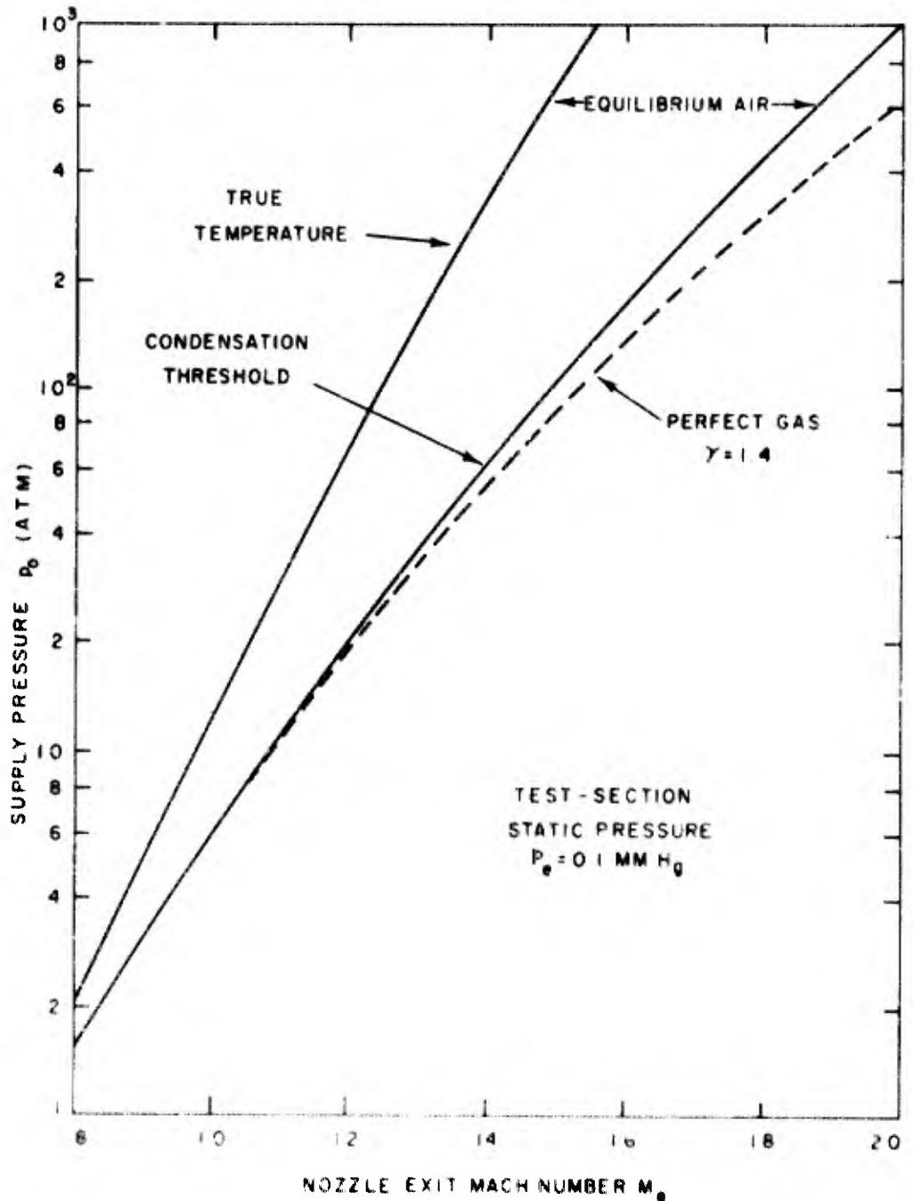
FIG 5 COMPARISON OF SUPPLY PRESSURE REQUIREMENTS
