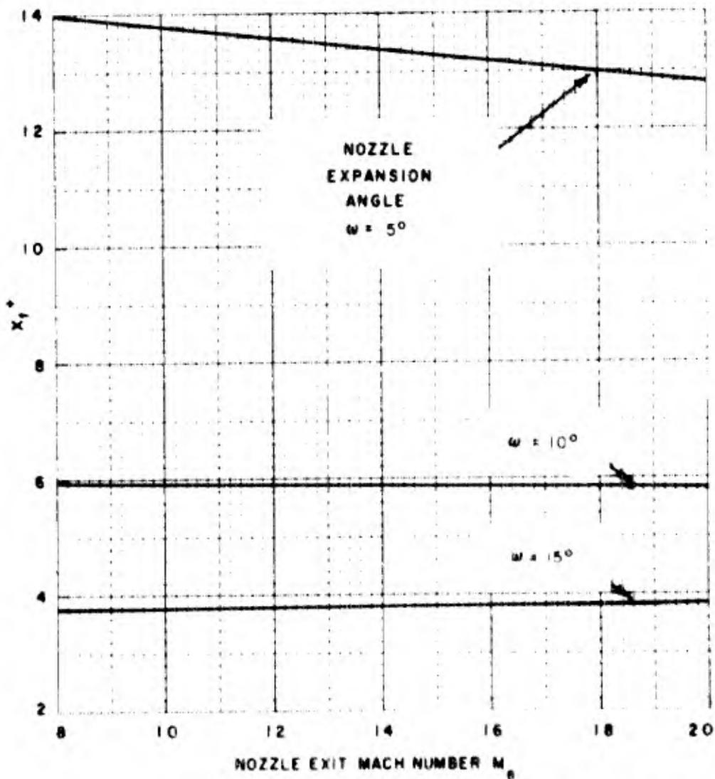
FIG 12 FOELSCH NOZZLE, DIMENSIONLESS LENGTH  $x_1^*$
