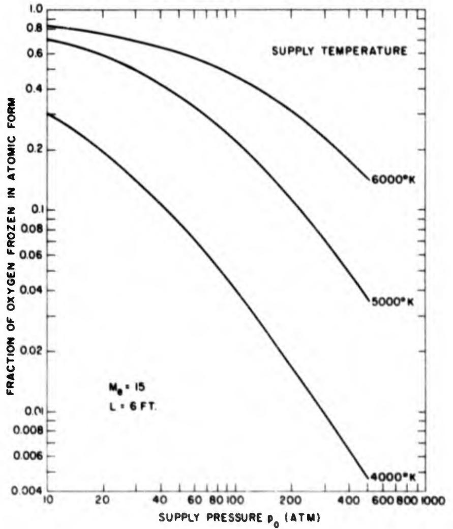
FIG 1 FRACTION OF OXYGEN FROZEN IN ATOMIC FORM IN A CONICAL NOZZLE
