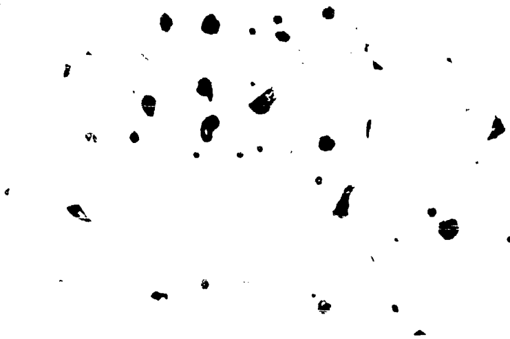
Figure 23a. A. R. \text{ZrB}_{1.96} Fired at 2100^{\circ}\text{C} for 6 hours 400X, Unetched.
