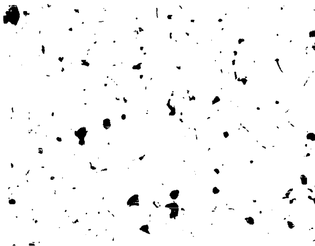
Figure 16a. FEM ZrB 1.89 Fired at 2300°C for 32 Minutes; (400X, Unetched).
