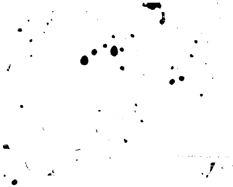
Figure 21a. FEM ZrB_{1.89} Fired at 2200^{\circ}C for 4 hours 400X, Unetched.
