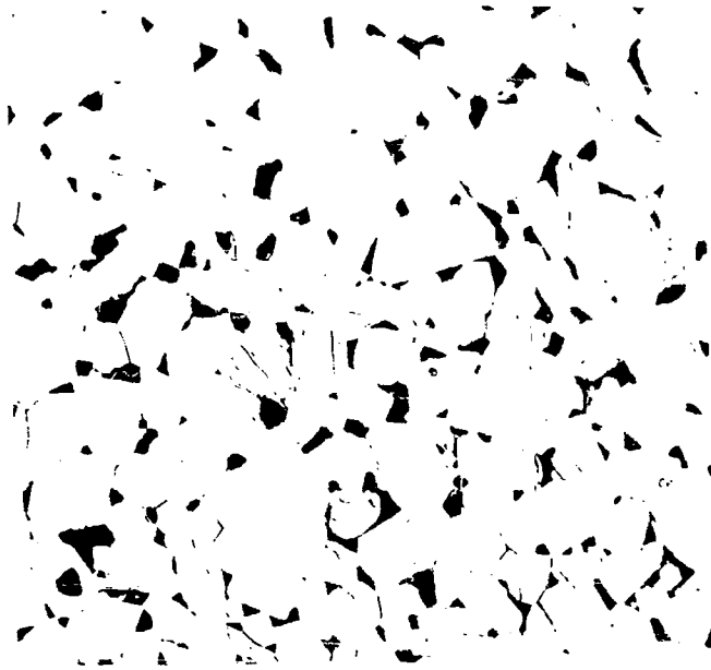
Etched X500 Etchant: Modified Aqua Regia High Pressure Hot Pressed, R-75 Fabricated from U. S. Borax TiB_2(1) .
