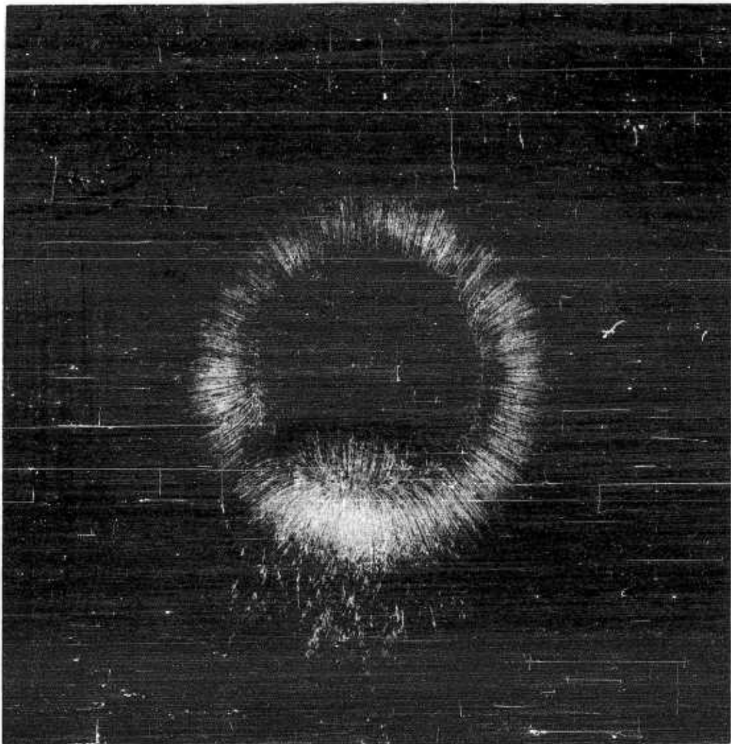
Figure 62. Typical grease streak photograph of flow pattern due to impingement on flat plate. p_1/p_\infty = 3.57 ; x/d_N = 5.32 .
