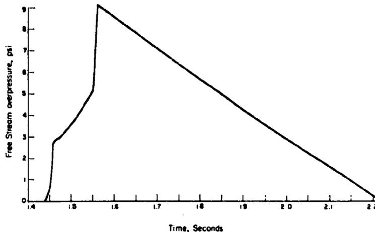
Figure 3.6 Estimated surface overpressure versus time variation at 3,500-foot ground range.
