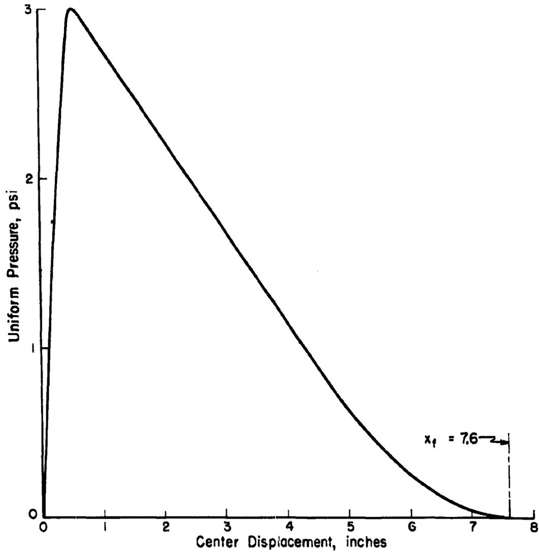
Figure 7.7 Predicted static resistance function for cinder block panel.
