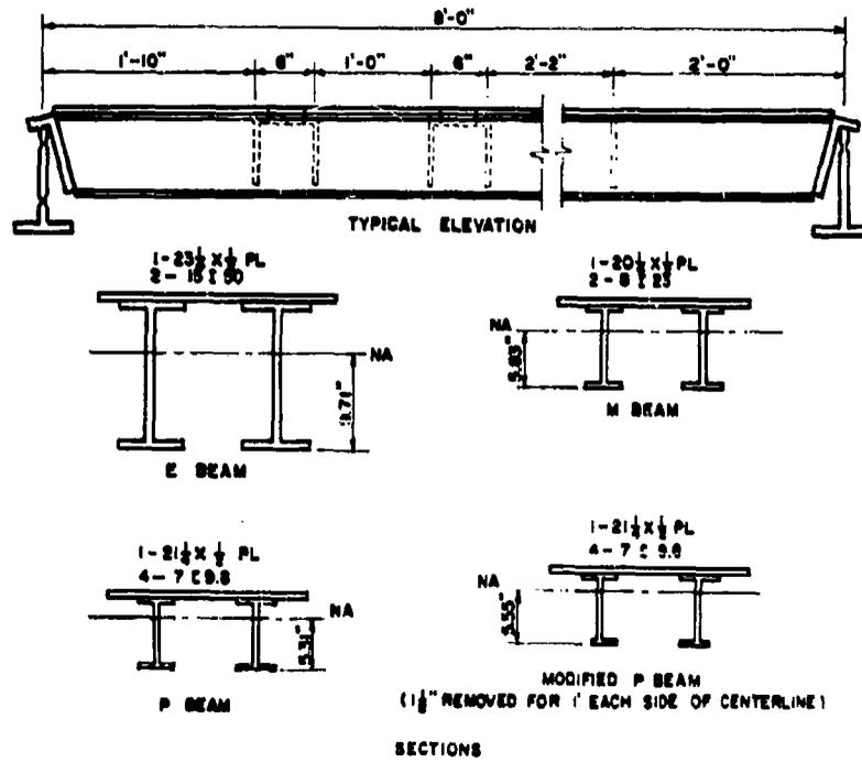
Figure 4.2 Details of typical UK 3.8 test beams.
