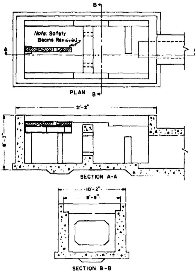
Figure 4.1 Details of typical UK 3.8 test structure.
