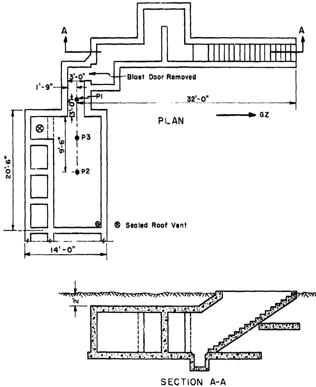
Figure 5.1 Details of UK 3.7 test chamber and location of pressure gages.
