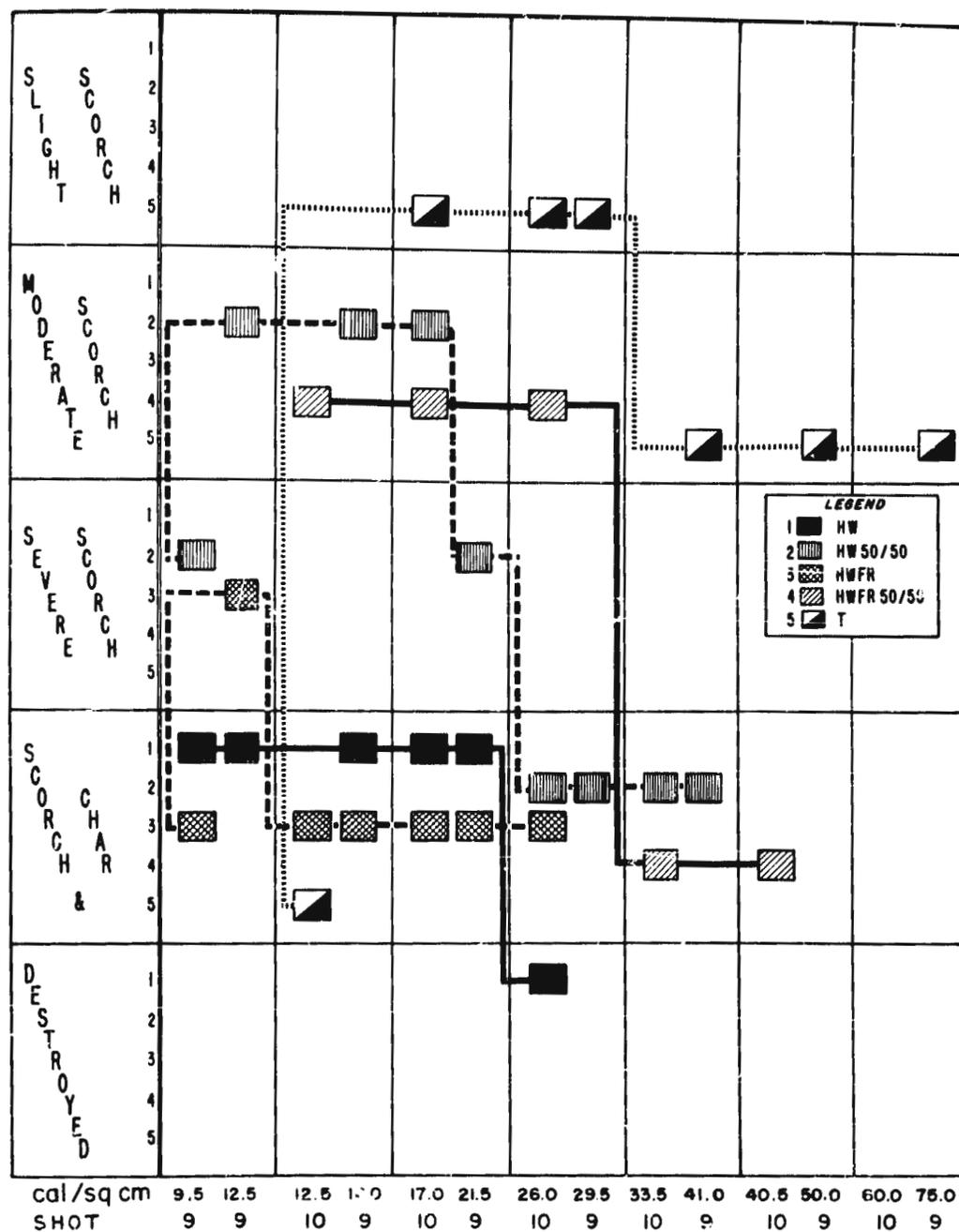
Fig. 2.1 Visual Evidence of Damage Sustained by Second Layers of Hot-Wet and Temperate Assemblies
