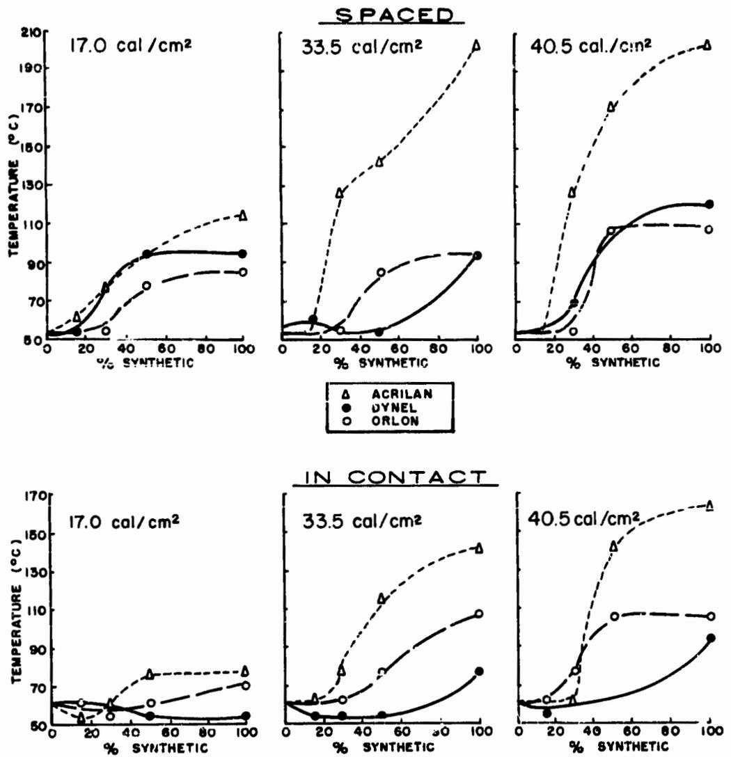
Fig. 3.1 Temperatures Attained under Wool Synthetic Blended Serges
