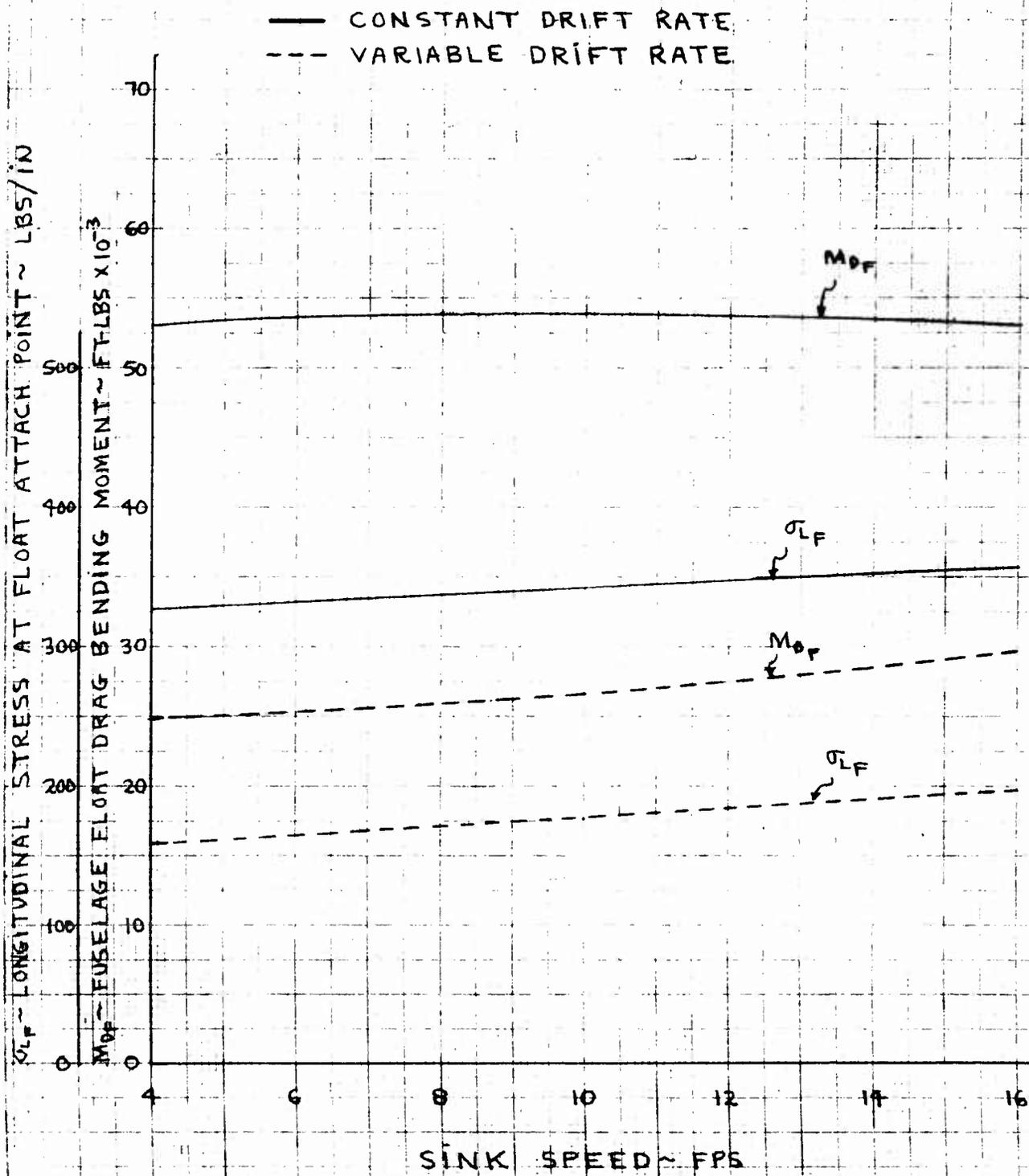
Figure 28 - Fuselage Float Drag Loads for Shorter Floats
