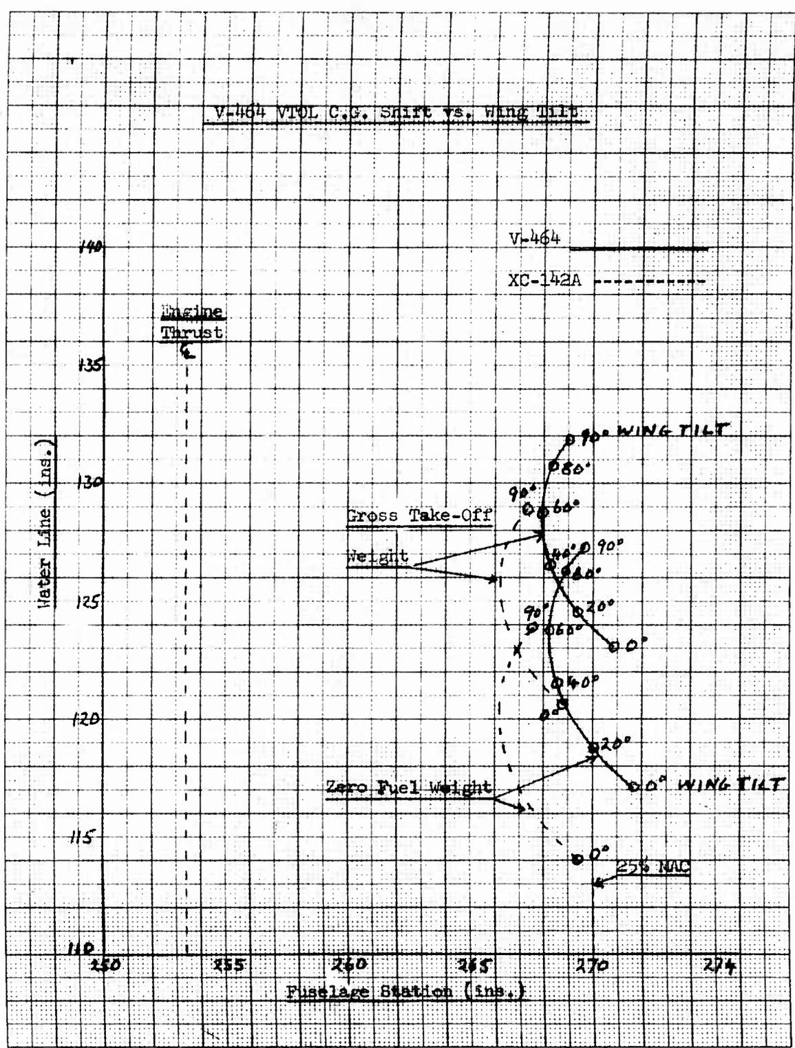
Figure 63 - VTOL V-464 Center of Gravity Shift vs Wing Tilt
