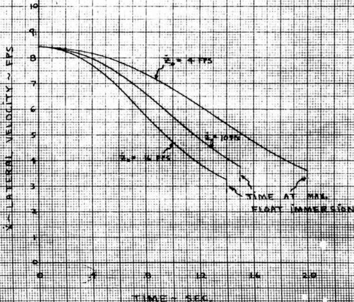
Figure 23 - Relative Velocity Between Airplane and Water During
