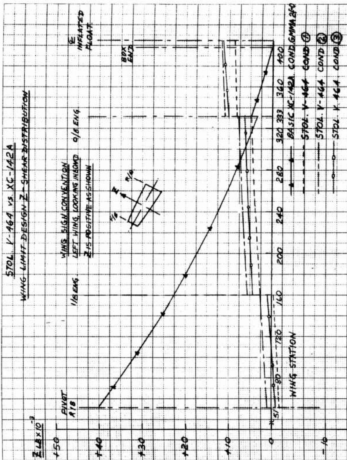
Figure 33 - STOL V-464 vs XC-142A Wing Limit Design; Z - Shear Distribution
