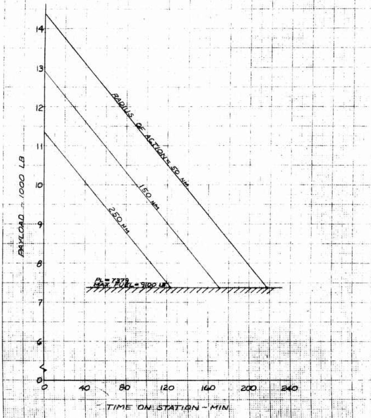
Figure 49 - STOL V-464 Payload vs Time on Station
