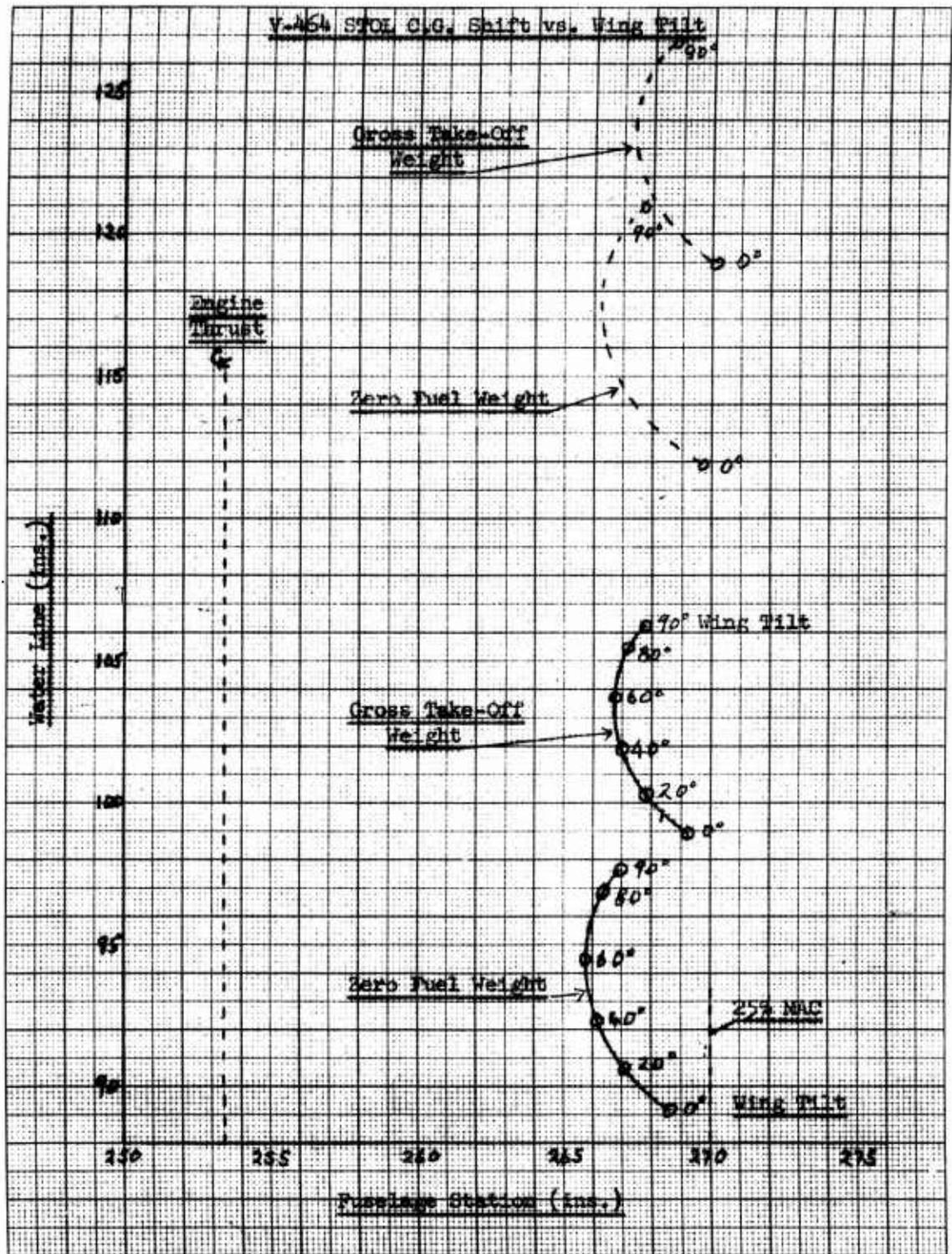
Figure 64 - STOL V-464 Center of Gravity vs Wing Tilt
