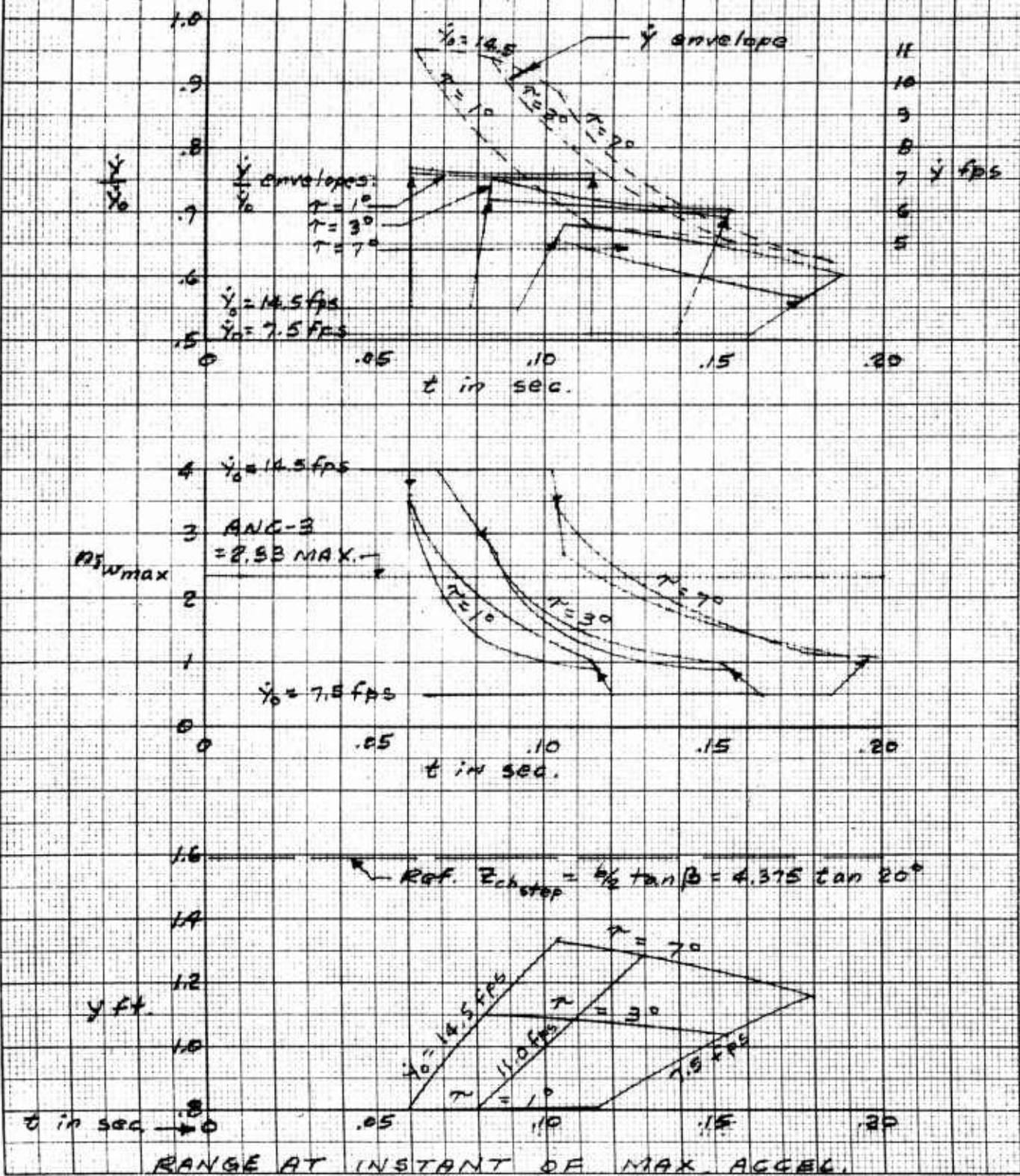
Figure 16 - STOL V-464 Hull Impact; parametric envelopes.
