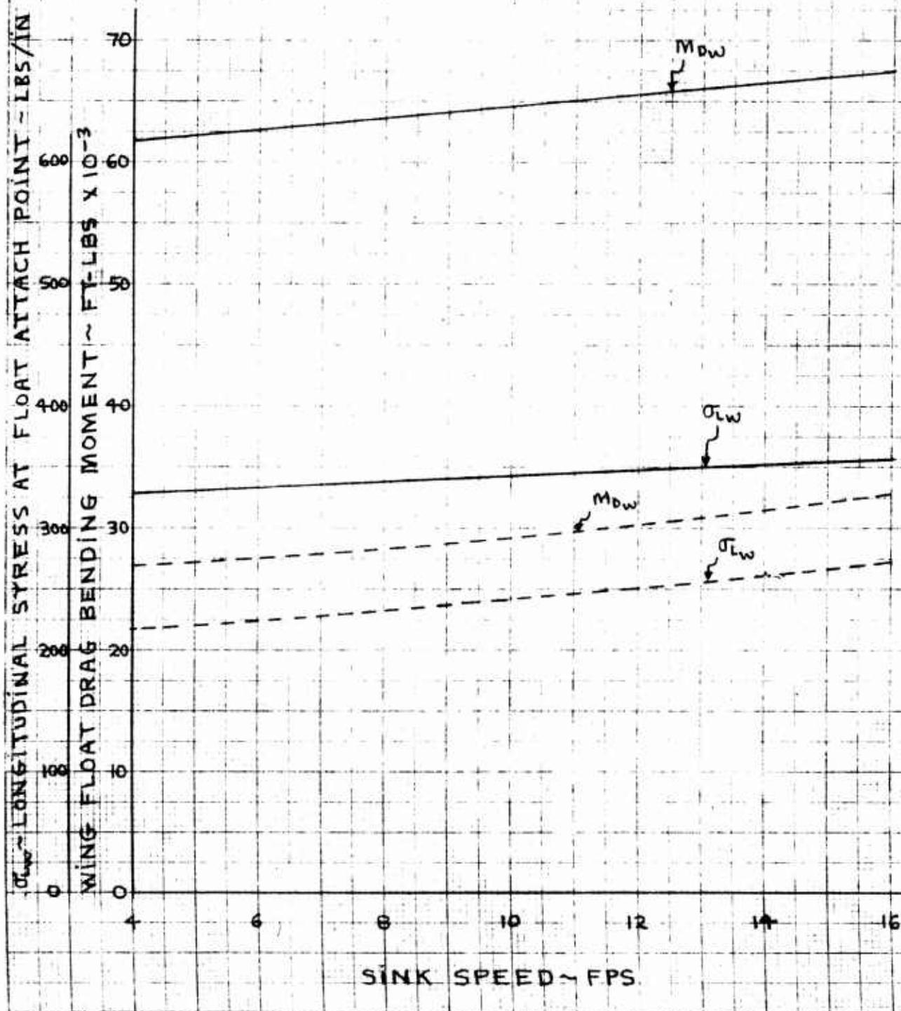
Figure 29 - Wing Float Drag Loads for Shorter Floats
