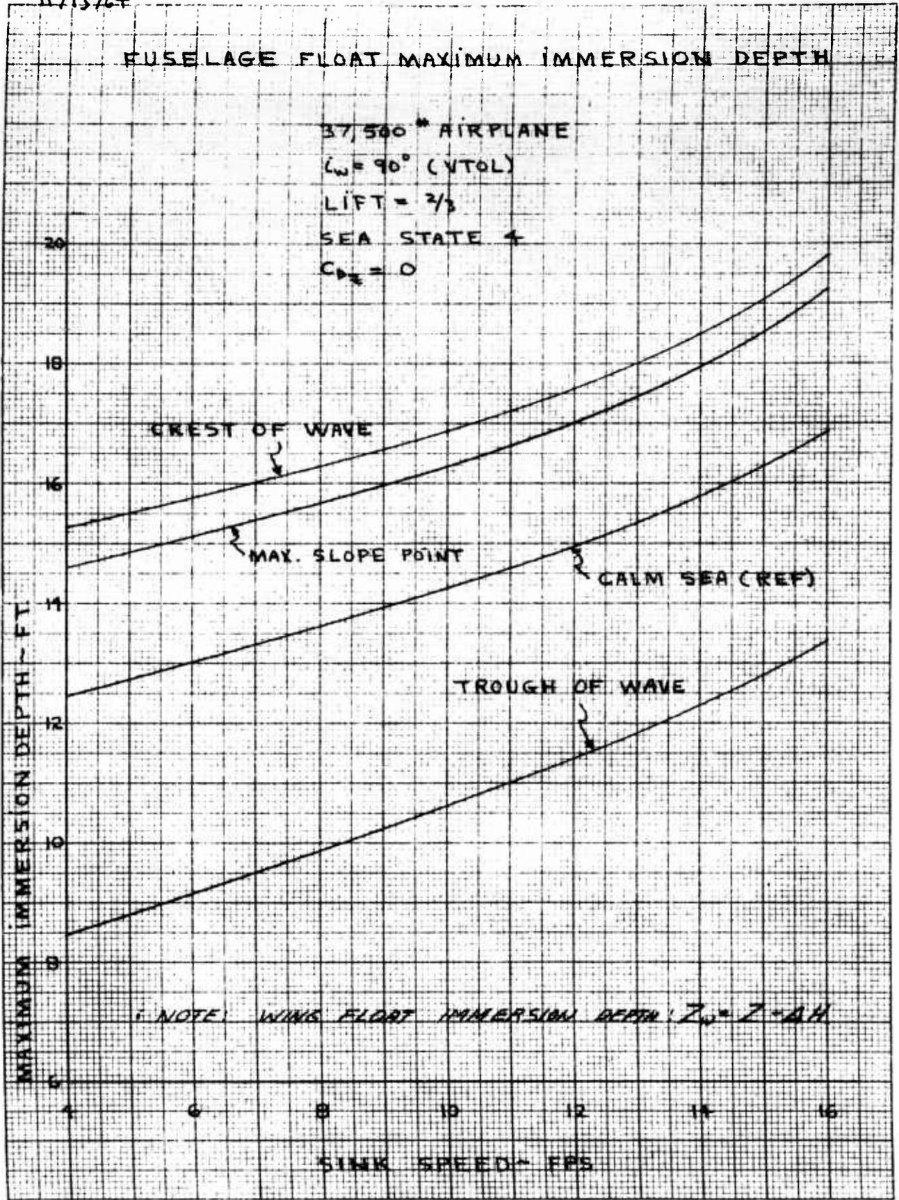
Figure 19 - Fuselage Float Maximum Immersion Depth
