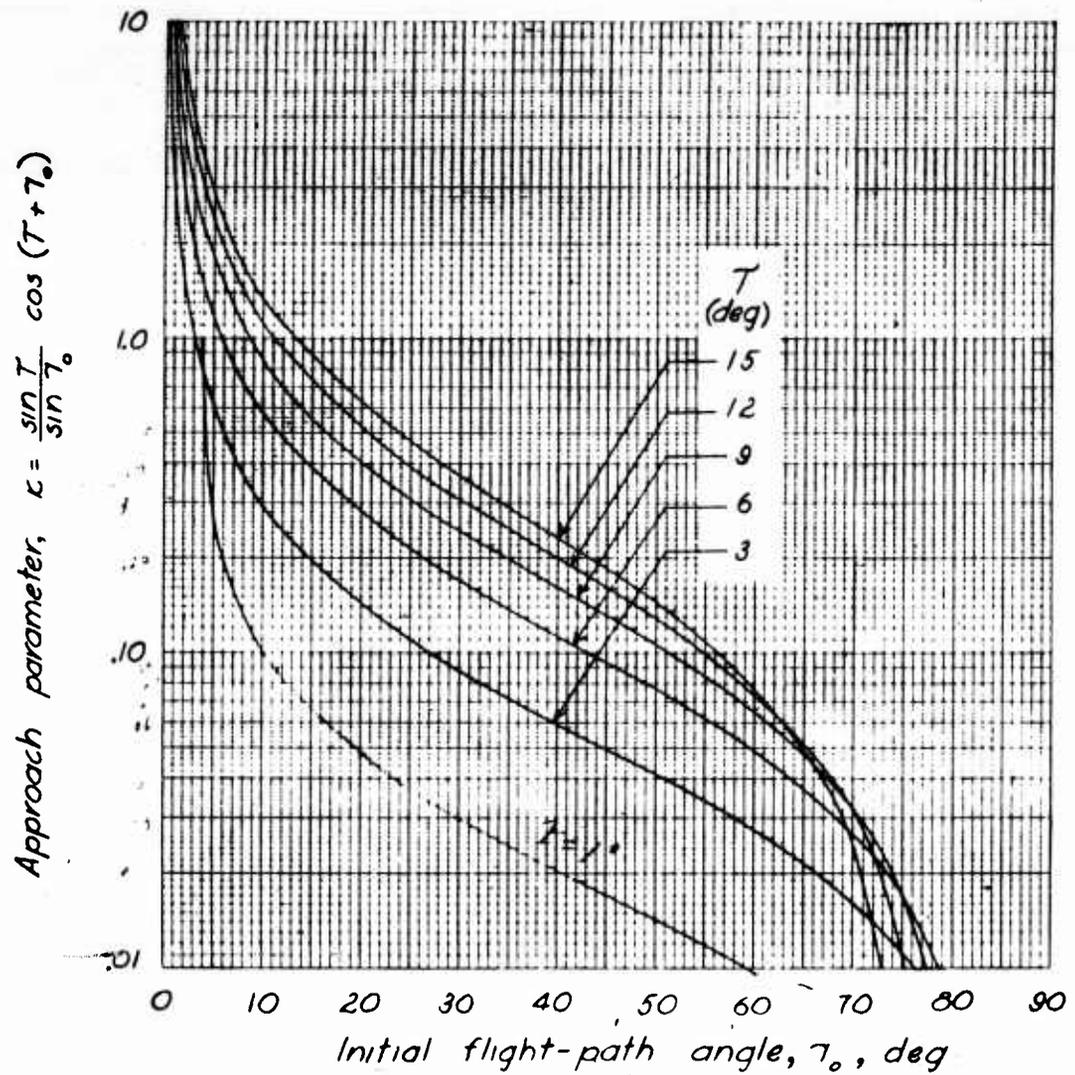
Figure 2. — Variation of approach parameter with trim and flight-path angle.
