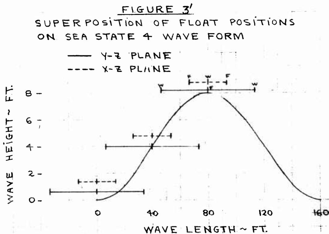
The relative water penetration into the wave form of the fuselage and wing floats can be scaled off of the figure. The fuselage floats are longer than the wing floats and strike the water first. The impact analysis has two parts: (1) fuselage float penetration up to the point where wing floats touch and (2) motion after all floats submerge.
