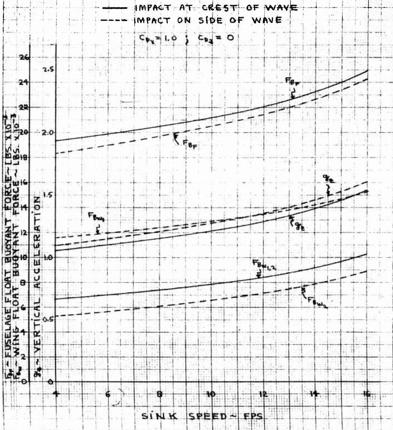
Figure 22 - Maximum Float Buoyant Forces and Resulting Maximum
