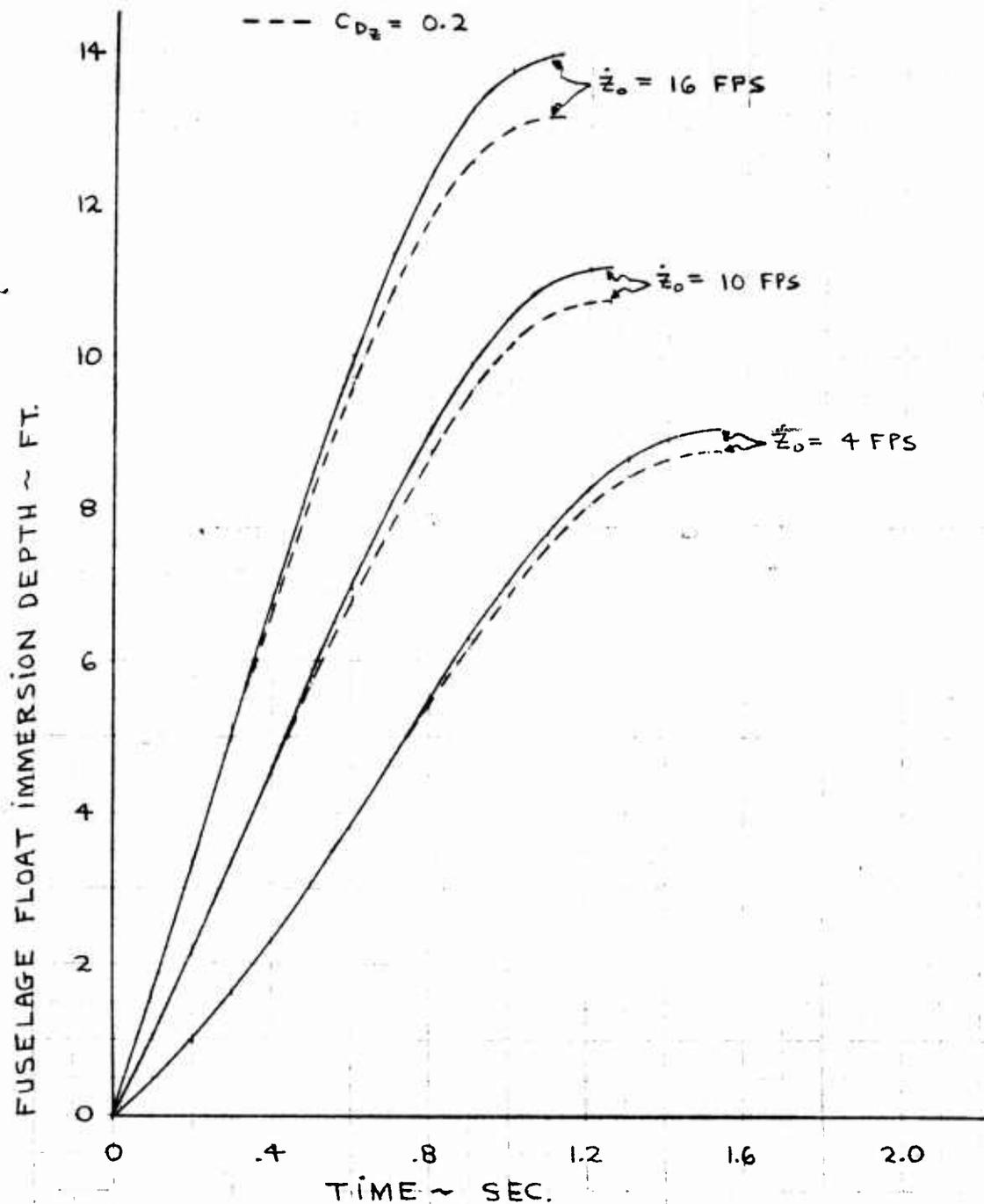
Figure 18 - Fuselage Float Immersion as a Function of Vertical Drag on Float
