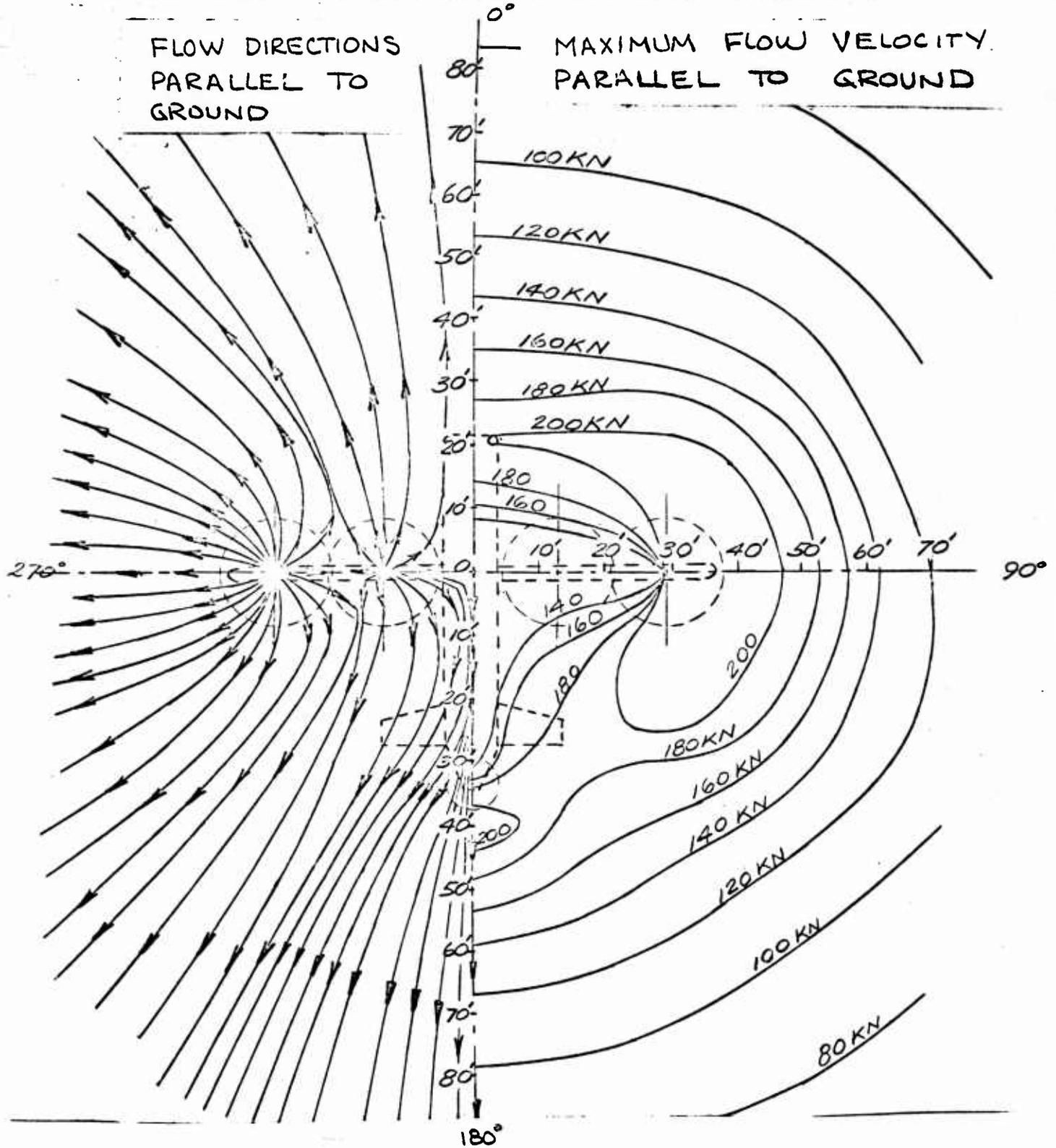
Figure 53 - Downwash Flow Along the Ground
