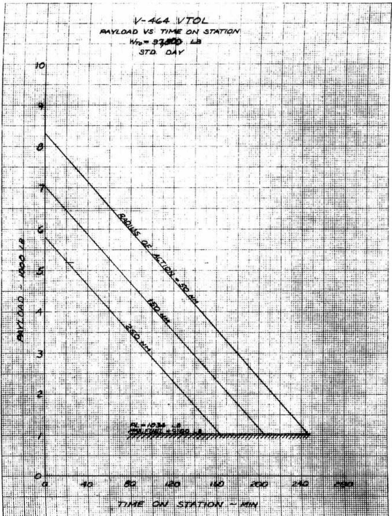
Figure 52 - VTOL V-464 Payload vs Time on Station
