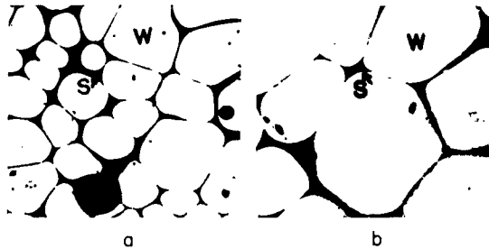
FIGURE 21. Grain Growth in poly-phase microstructures. Example: Wüstite (FeO) growth in an iron oxide saturated silicate liquid (approx. X84). (a) Four hours at 1200°C (2190°F). (b) 64 hours at 1200°C [19]. W - wüstite; S - silicate liquid.
