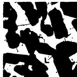
FIGURE 28. Solid contact. Example: cristobalite ( \text{SiO}_2 ) and a silica-saturated iron oxide liquid (X169). Although more than 25 percent liquid is present, a large dihedral angle (fig. 11b) provides solid-to-solid contact and structural rigidity at high temperatures. (Cf. fig. 27 and fig. 2b.) C - cristobalite; L - silicate glass.
