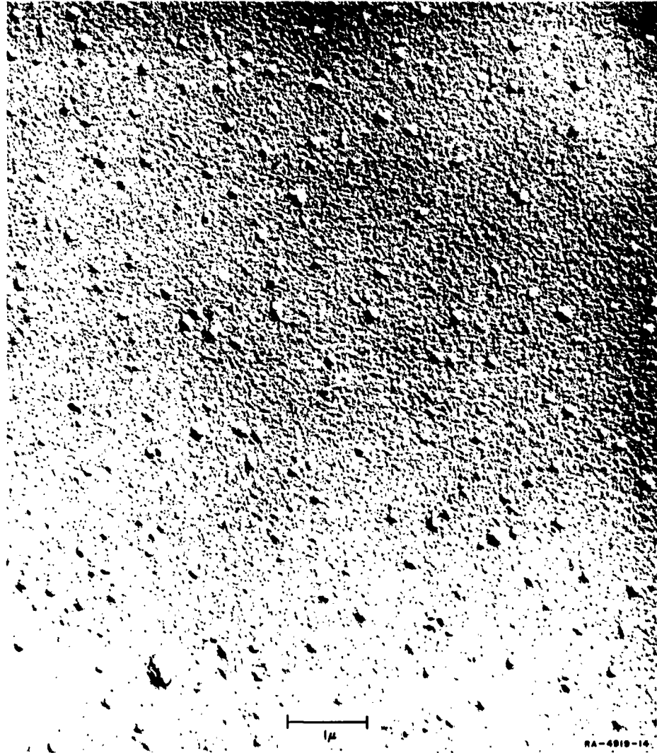
FIG. 2 SURFACE REPLICA OF ALUMINUM FILM DEPOSITED ON SUBSTRATE AT ROOM TEMPERATURE
