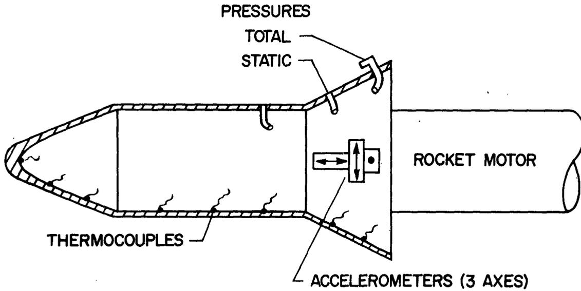
Fig.4 Telemetered measurements
