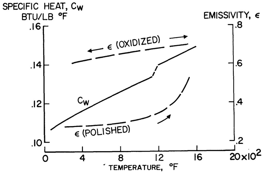
Fig.7 Specific heat and emissivity of Inconel
