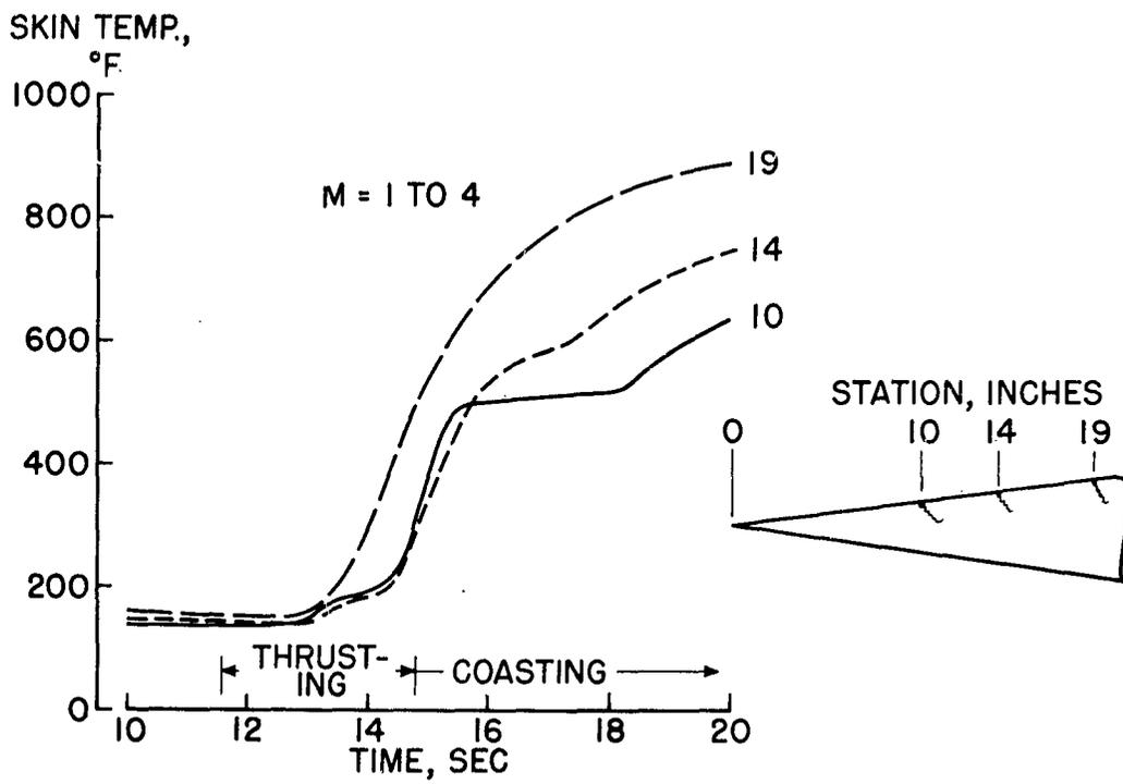
Fig.8 Temperatures measured on a thermally thin skin
