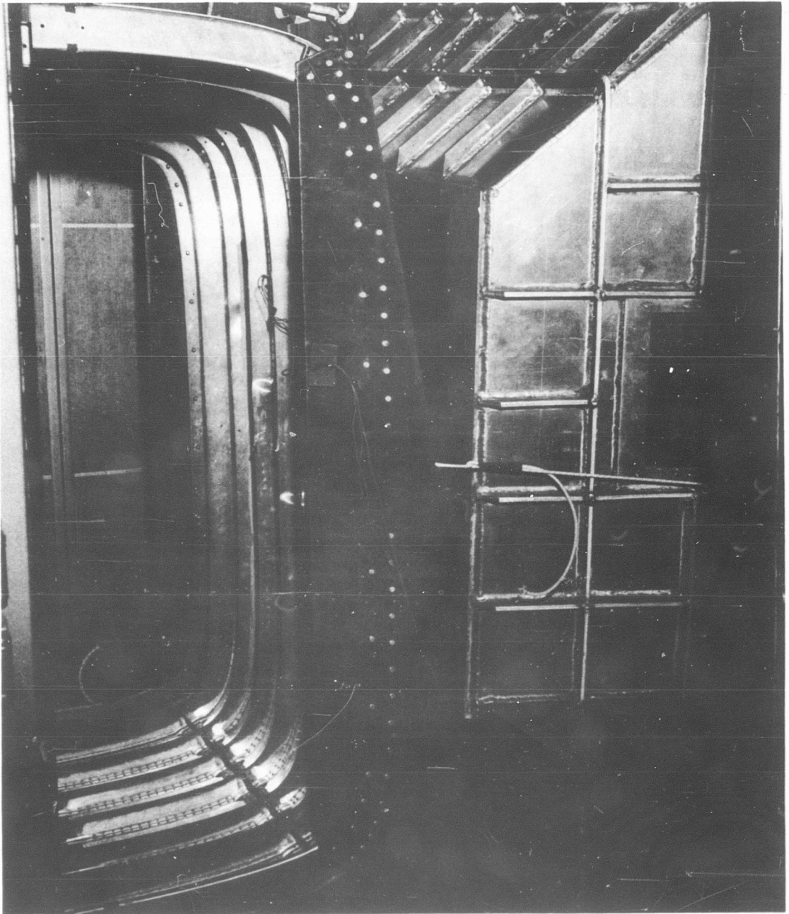
Figure 6. Arrangement for the Measurement of Sound Induced Vibrations - Fuselage Specimen on Left
