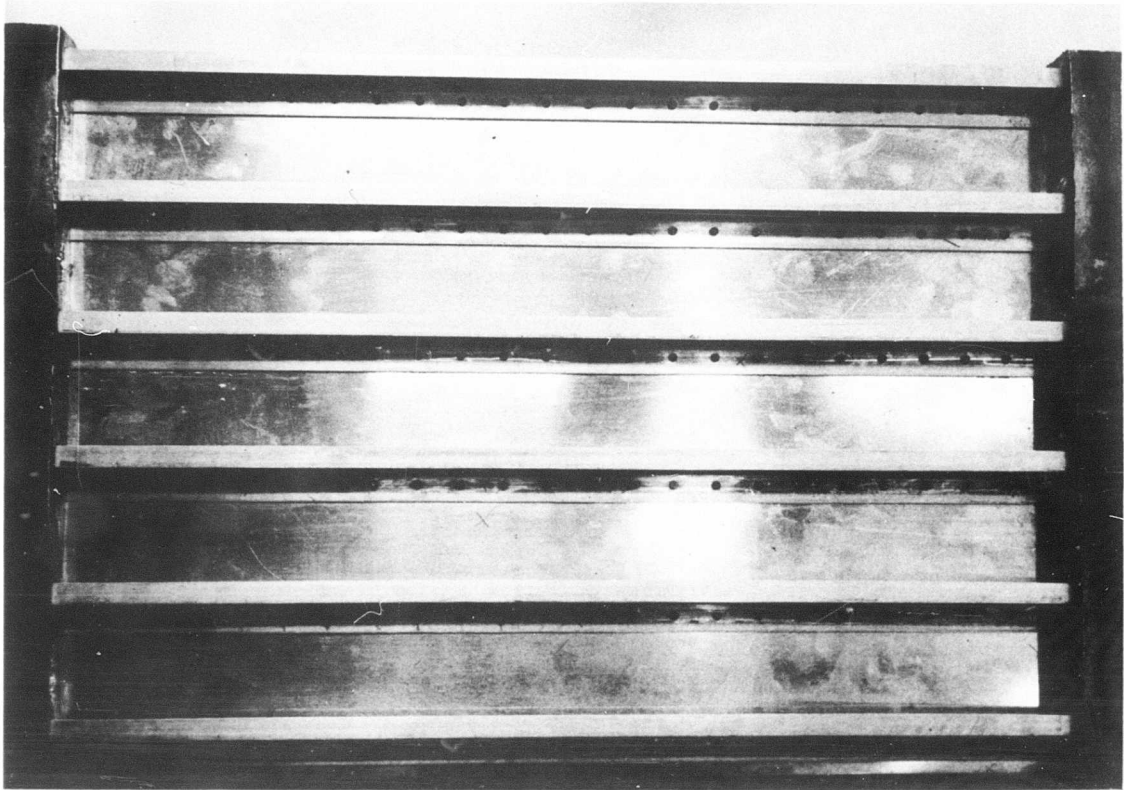
Figure 6. Wing Compression Test Panel - Bottom View
