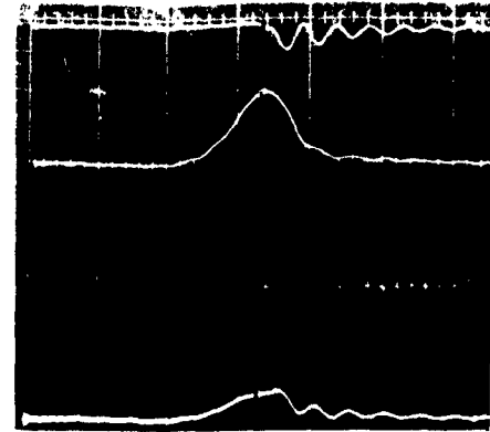
Upper Trace: Monitor Signal Vertical Sensitivity Middle Trace: Return Signal (Antenna Port) Vertical Sensitivity Lower Trace: Receiver Return Signal Vertical Sensitivity Horizontal Sweep Sp
