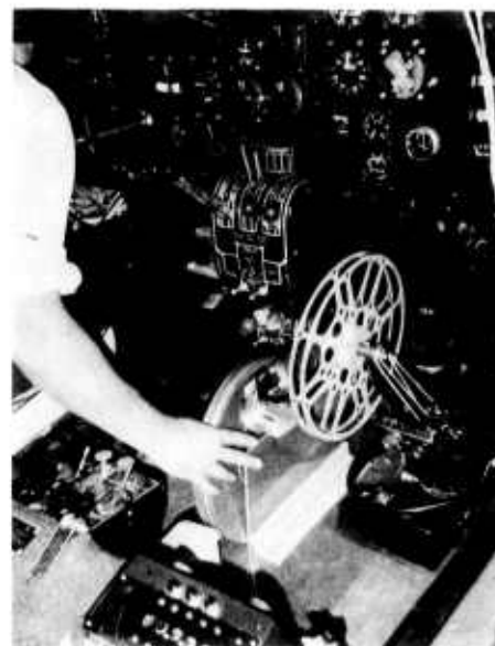
Projector drive system, with enclosed supply reel and take- up reel.
