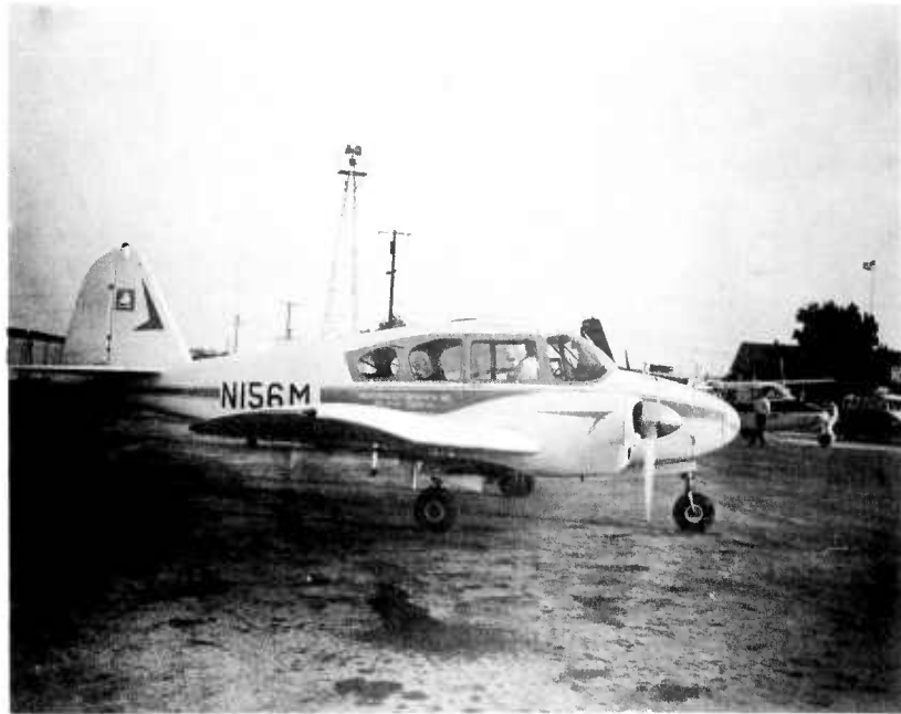
a. Supercharged Piper Apache. The potential gradient probes can be seen above and below the fuselage. Sampler not yet installed at nose.
