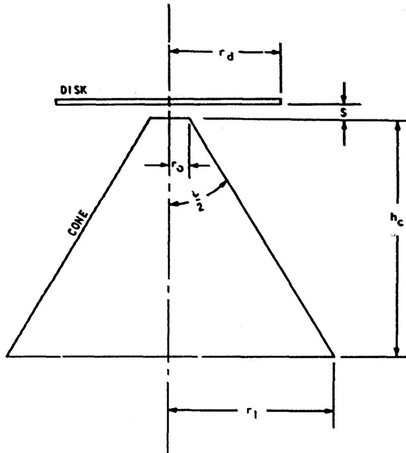
Figure 1. Discose Geometry.
