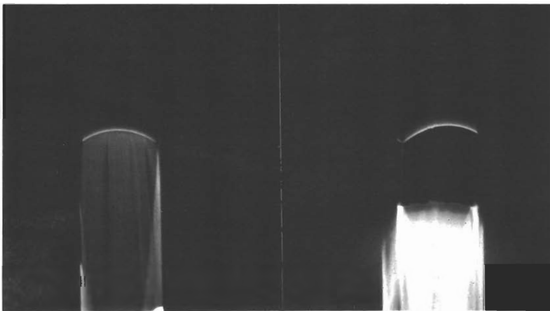
Fig. 8 RMC trace of detonations emerging from charges of RDX at 60% of crystal density. The charge on the left is at 580 torr while that at right is at a few microns.
