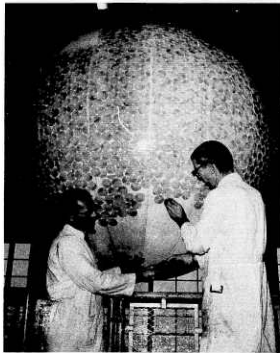
Fig. 3. Technique for applying foam pellets to balloon surface.
