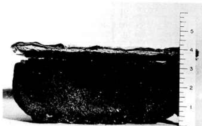
Fig. 2. Photograph of composite sheet and cross section through a foamed layer.
