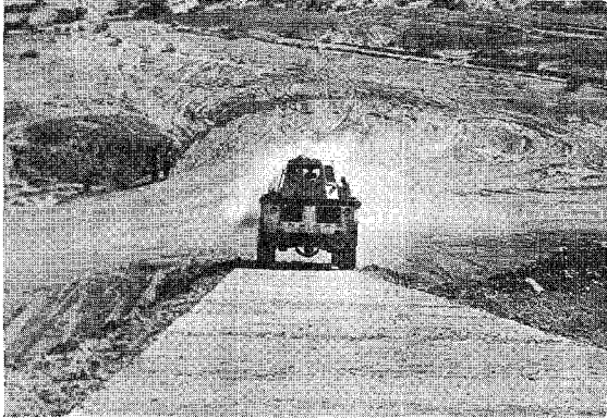
Figure 116. Lighter Negotiating 40-Percent Paved Grade--Normal Land Drive.
