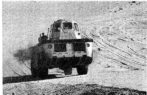
Figure 119. Lighter Negotiating 30-Percent Sand Grade.
