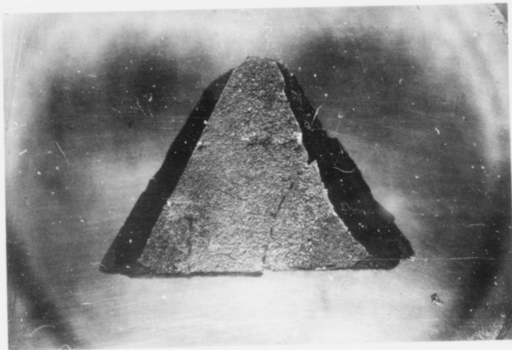
Figure 4. Photograph of a cross section of the #3 pressed oxide powder tetrahedron. Corners of cross section show some darkening and general texture is somewhat rough; density 3.52. Original magnification 8 x
